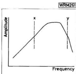
Fig. 3.4: Typical i.f. response of a conventional TV receiver
