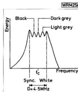
**Fig. 3.1: Energy distribution of a simple grey scale**
