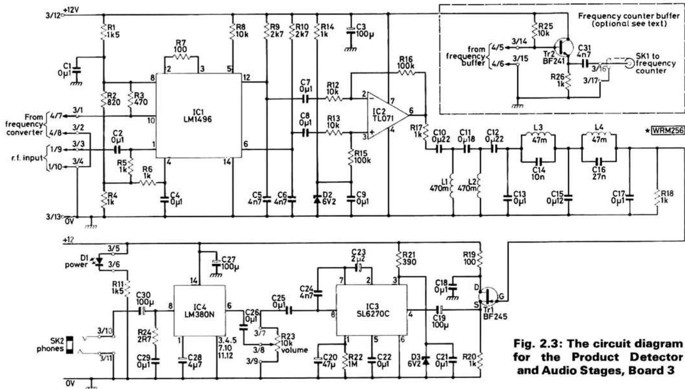
**Fig. 2.3: The circuit diagram for the Product Detector and Audio Stages, Board 3**
