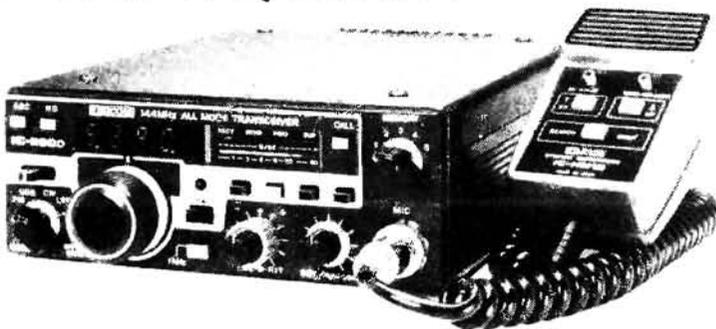
290D is the state of the art 2 meter mobile, it has 5 memories and VFO's to store your favourite repeaters and a priority channel to check your most important frequency automatically. Programmable offsets are included for odd repeater splits, tuning is 5KHz or 1KHz.
