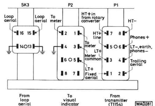
Fig. 3: Connectors as seen looking at the front panel of the R1155
