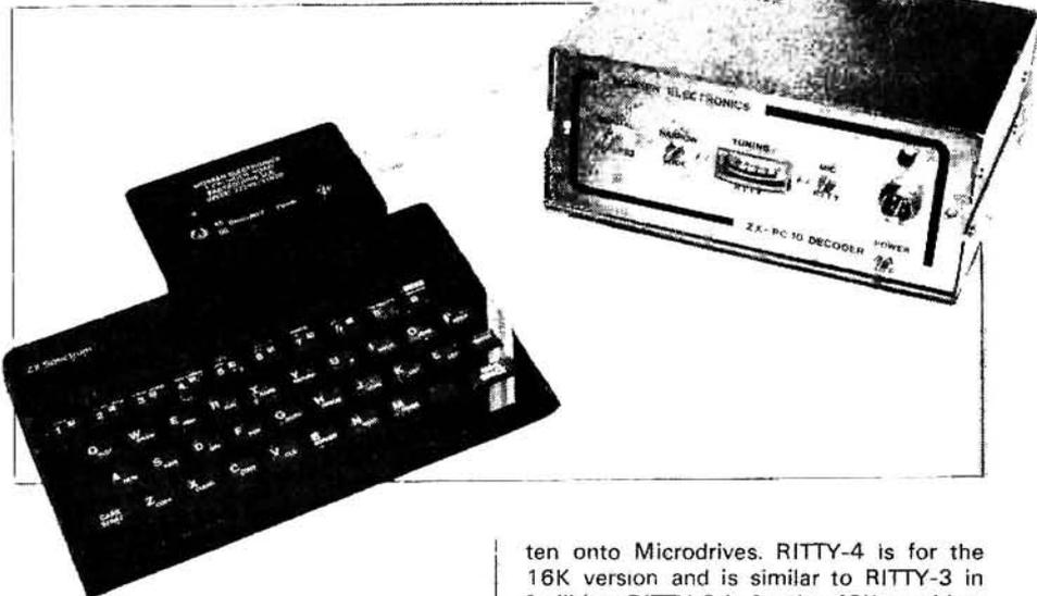
ZX81—RITTY-2 and 3 are supplied in EPROM form with your callsign programmed into the CQ call routine. Both have full transmit and receive capability but RITTY-3 is more advanced than RITTY-2 with 26 programmable stores plus 2 pre-programmed stores. It also uses a split screen, type ahead and can output to a ZX Printer.
