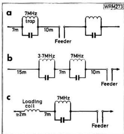
**Fig. 1: (a) Approximate dimensions of trapped dipole covering 3.5 to 28MHz, fed with low impedance coaxial cable. (b) Same as (a) but with additional traps at 3.7MHz and end wires but now extending coverage to 1.8MHz. (c) The use of a loading coil instead of a trap considerably reduces length of end wires for coverage of the h.f. and l.f. bands**
