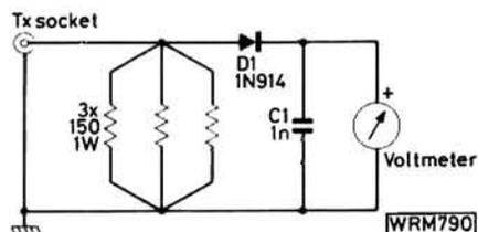
**Fig. 1: Suitable circuit for low power measurement in a 50Ω system. The resistors should not be wirewound. All leads (except those to voltmeter) should be as short as possible (10mm maximum). The meter will read  $(\sqrt{100P})-0.6$  volts for a power of P watts (16.7V at 3 watts)**
