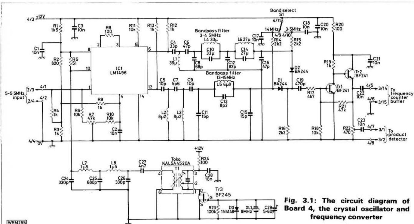
Fig. 3.1: The circuit diagram of Board 4, the crystal oscillator and frequency converter
