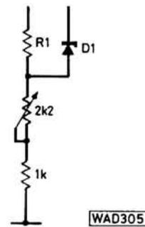
**Fig. 3: A circuit modification that can be incorporated, replacing R2 to give adjustable voltage cut-off**
