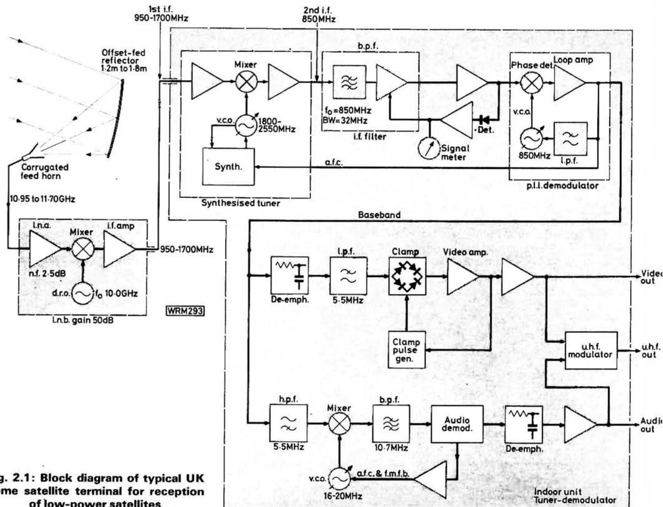
Fig. 2.1: Block diagram of typical UK home satellite terminal for reception of low-power satellites
