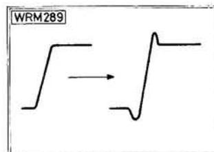
Notches and peaks in the video frequency response can have strange effects, e.g. loss of colour on a seemingly perfect full bandwidth signal—due to a notch at 4.43MHz. One common distortion deliberately introduced is high-frequency boost in a signal which has been bandwidth limited, e.g. the 3MHz bandwidth signal in a v.c.r. The effect of a boost at the h.f. end is to increase the visual sharpness of edges; however if it is overdone the edges "ring" and noise increases too, Fig. 4.7.
