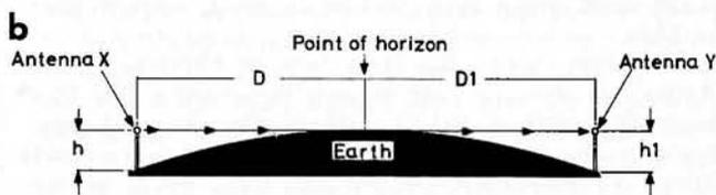
Fig. 6.1: (a) A v.h.f./u.h.f. wave may reach a distant antenna via reflection from ground to combine with the direct antenna to antenna signal (see text) (b) Horizon to horizon distance versus height of transmitting and receiving antennas (see text)
