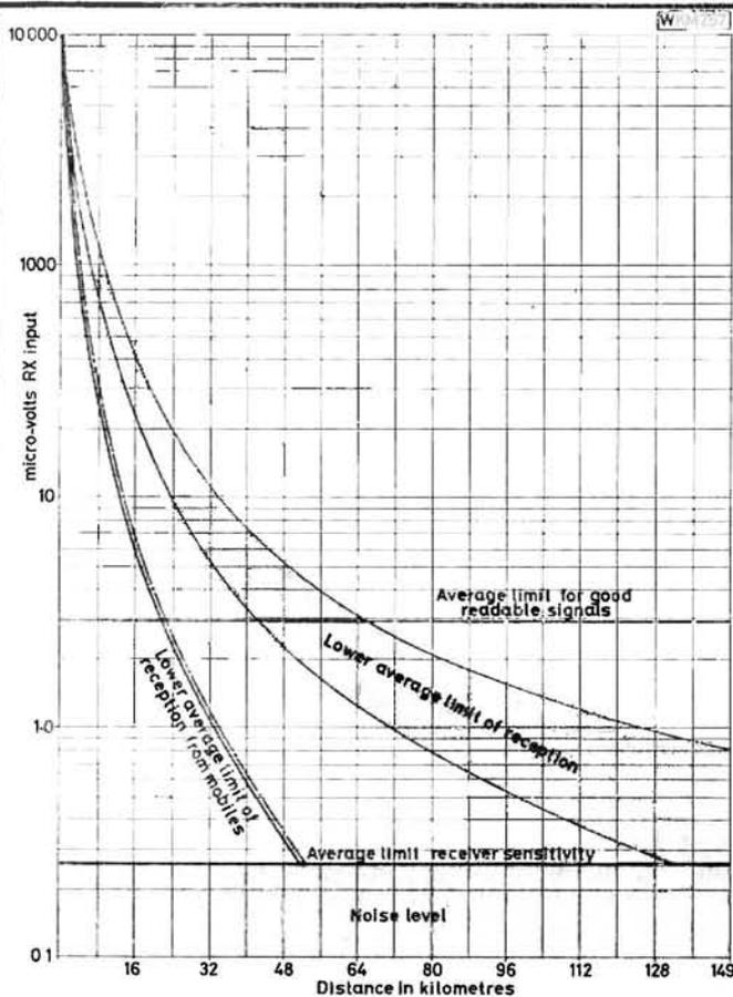
**Fig. 6.4: Average signal level versus distance; fixed station to fixed station and fixed station to mobiles. Note: Distance may be limited by receiver sensitivity, transmitter power and type of antenna in use. Curves relate to vertically polarised transmissions**
