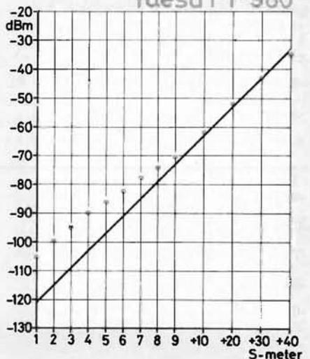
is a part-kit transceiver which I built, and the S-meter calibration control was set up on the basis that a signal that I judged subjectively to be an S1 just didn't move the meter needle off
