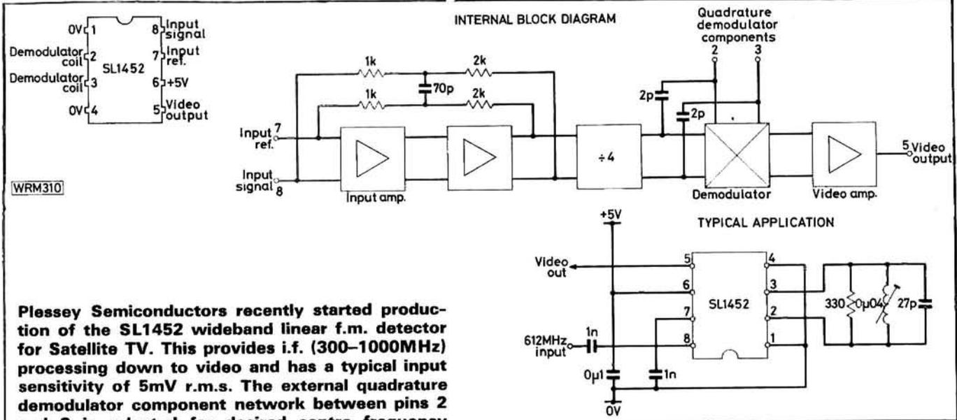
**Plessey Semiconductors recently started production of the SL1452 wideband linear f.m. detector for Satellite TV. This provides i.f. (300-1000MHz) processing down to video and has a typical input sensitivity of 5mV r.m.s. The external quadrature demodulator component network between pins 2 and 3 is selected for desired centre frequency bandwidth**
