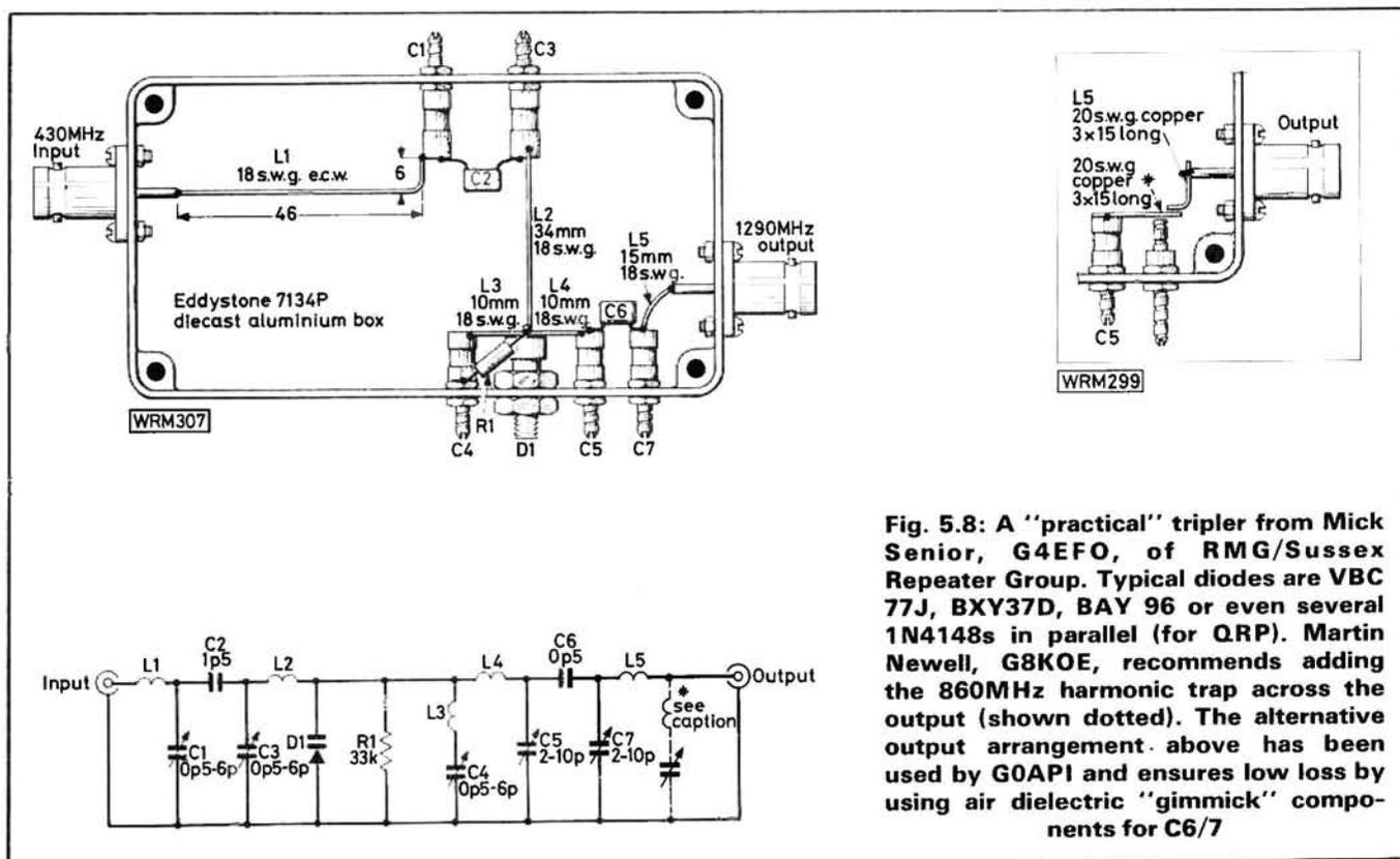
**Fig. 5.8: A "practical" tripler from Mick Senior, G4EFO, of RMG/Sussex Repeater Group. Typical diodes are VBC 77J, BXY37D, BAY 96 or even several 1N4148s in parallel (for QRP). Martin Newell, G8KOE, recommends adding the 860MHz harmonic trap across the output (shown dotted). The alternative output arrangement above has been used by G0API and ensures low loss by using air dielectric "gimmick" components for C6/7**
