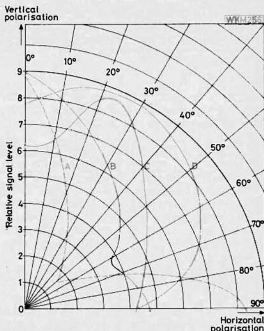
Fig. 6.3: Variations in polarisation from four stations each using vertically polarised antennas (see text)
