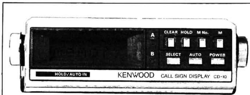
**The CD-10 callsign display decodes and displays digital data input as audio. Up to 20 callsigns can be held in its memory or interfaced with your micro for log keeping**
