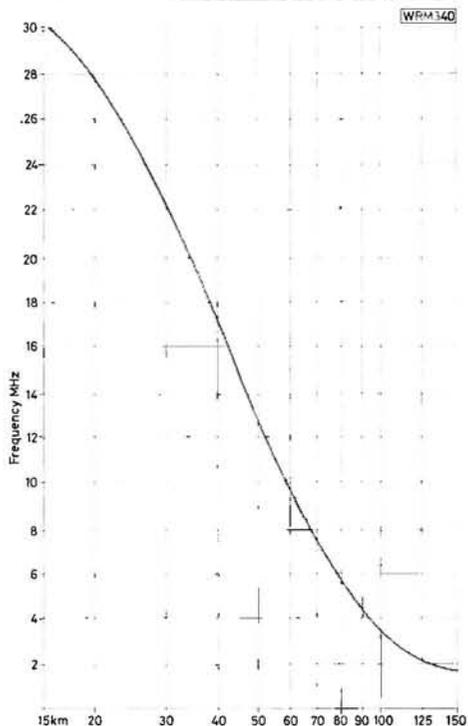
**Fig. 8.4: Ground range versus frequency for groundwave propagation. (Daytime conditions 2 to 30MHz)**
