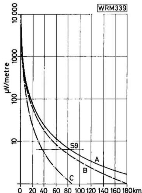
Fig. 8.3: Groundwave field strength at 1.8MHz based on the Sommerfeld equation. (A) from a  $\frac{3}{8}$  vertical antenna. (B) from a well elevated horizontal  $\frac{1}{4}$  antenna. (C) from an "L" shaped antenna with most of the horizontal portion at low height. Note: These are for daytime conditions
