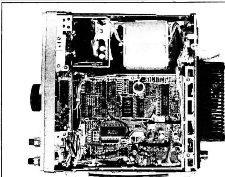
**An internal view of the TS-711E which indicates the extent of the circuit integration employed in current transceivers**
