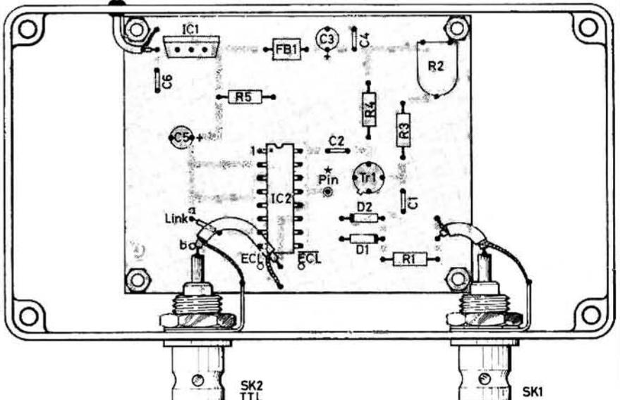
**Fig. 1: Full size p.c.b. layout and constructional details**
