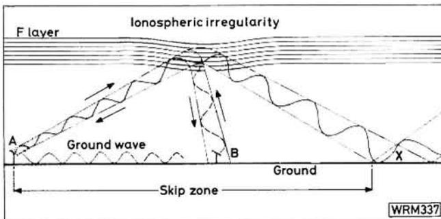
**Fig. 8.1:** Irregularities such as tilting in an ionospheric layer can cause scatter mode propagation so that signals from (A) arrive at some point (B) within a skip zone but which would otherwise only be heard at (X). Groundwave from (A) is too weak to reach point (B)
