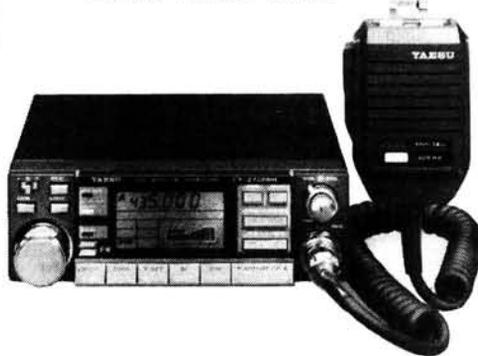
The FT2700R, virtually two transceivers in one case, is designed to be the ultimate in convenience, for FM mobile or base station operation, on the 144 and 430MHz bands. Using Yaesu's new one piece die-cast aluminium chassis concept, the FT2700R provides 25 Watts continuous output on either band, for full duplex (or simplex) operation whilst obtaining optimum circuit shielding and efficient heat dissipation.
