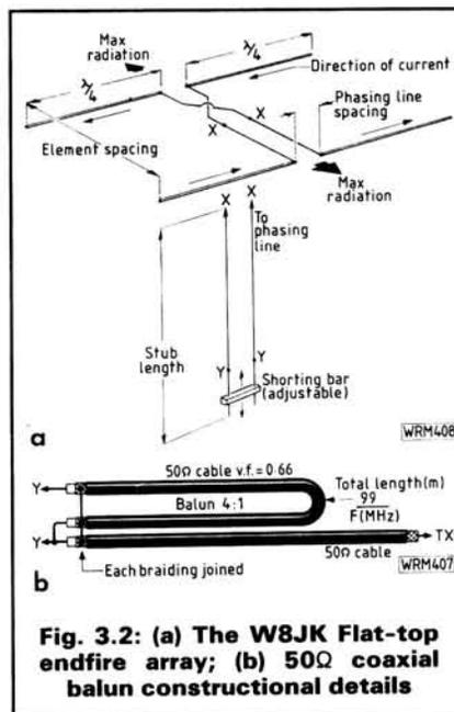
**Fig. 3.2:** (a) The W8JK Flat-top endfire array; (b) 50Ω coaxial balun constructional details
