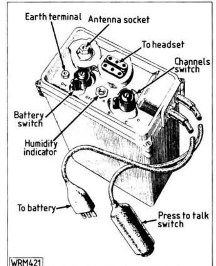
Fig. 2: The front panel of the No. 88 set ▶
