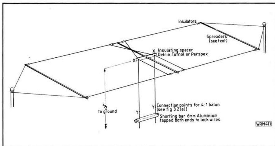
**Fig. 3.5: Suggested constructional details of the W8JK 2-element Flat-top beam**
