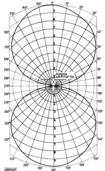
**Fig. 3.3:** The freespace horizontal radiation pattern of the W8JK 2-element Flat-top beam
