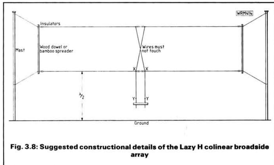
**Fig. 3.8: Suggested constructional details of the Lazy H colinear broadside array**
