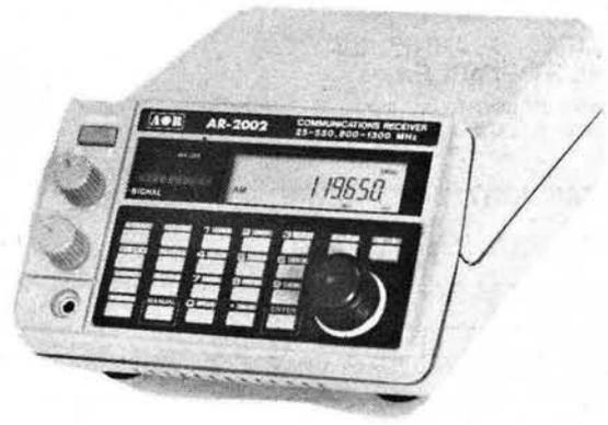
**Frequency range of the AR2002** is from 25 to 550 and from 800 to 1300 MHz. Modes of operation are wide band FM, narrow band FM and AM. The receiver has 20 memories, memory scan and a search mode which checks frequencies between user designated limits. The receiver has a push button keypad for easy frequency entry and operation.
