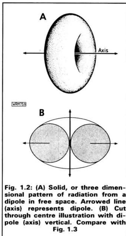
**Fig. 1.2: (A) Solid, or three dimensional pattern of radiation from a dipole in free space. Arrowed line (axis) represents dipole. (B) Cut through centre illustration with dipole (axis) vertical. Compare with Fig. 1.3**
