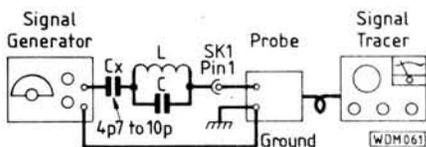
Fig. 6: Equipment layout showing probe connections used for resonance testing
