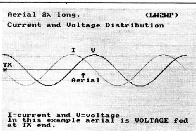
Fig. 4.1: Voltage and current distribution on a linear radiator 2 wavelengths long. (see text regarding harmonic operation)
