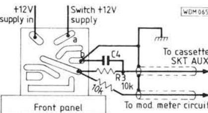
**Fig. 4: Connections to volume control p.c.b.**
