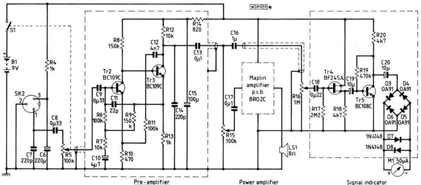
Fig. 1: Circuit diagram of amplifier and indicator
