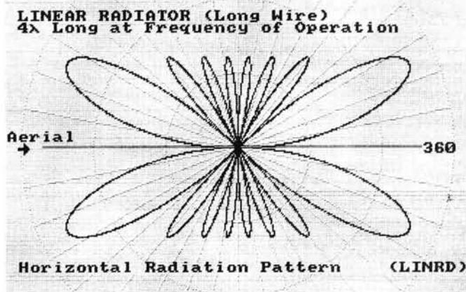
Fig. 4.4: Radiation pattern. Linear radiator 4 wavelengths long. Note number of minor lobes and that main lobes are at a smaller angle to the radiator. (see text)
