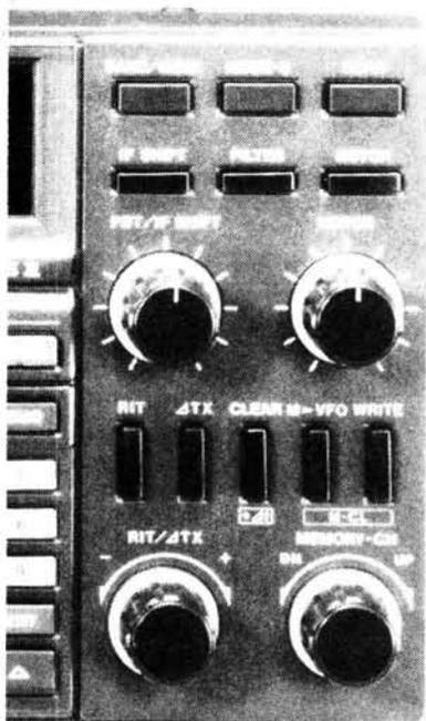
The new ICOM IC-761 H.F. Transceiver has many features making it probably the best top of the line Amateur transceiver available today. This all mode transceiver features an internal aerial tuning unit and A.C. power supply. The A.T.U. boasts a 3 second band selection and tune up with a VSWR matching of less than 1.3:1.
