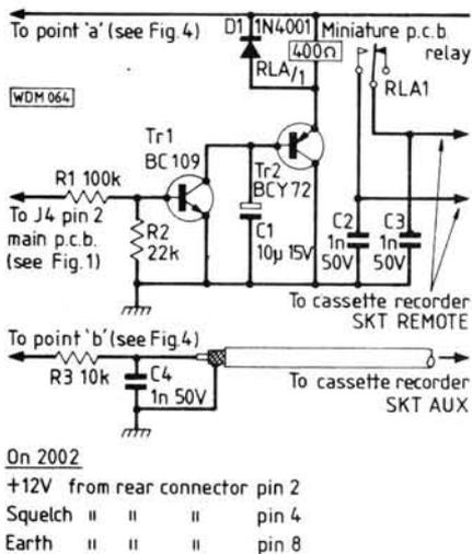
**Fig. 3: Cassette recorder interface circuit**
