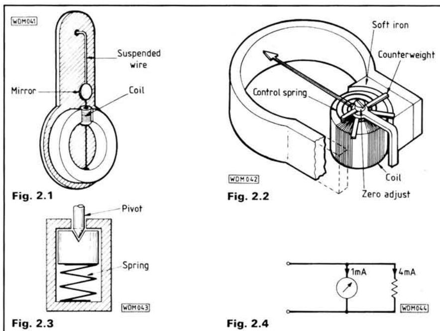
phor bronze springs of uniform thickness and precision manufacture to prevent kinking during use. The needle also has three weights. These counter weights are adjusted in the factory for accurate deflection at various readings. The moving parts pivot on an Incabloc assembly similar to that used by watch manufacturers, Fig. 2.3. Any shocks to moving parts are absorbed by the spring in the Incabloc.
