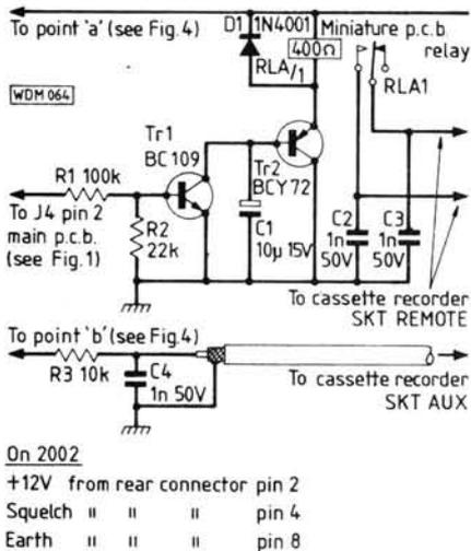
**Fig. 3: Cassette recorder interface circuit**
