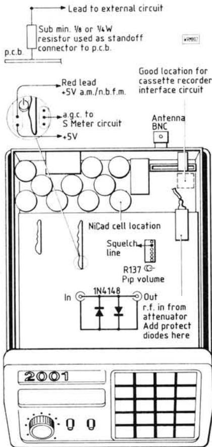
Fig. 1: Internal layout of AR-2001
