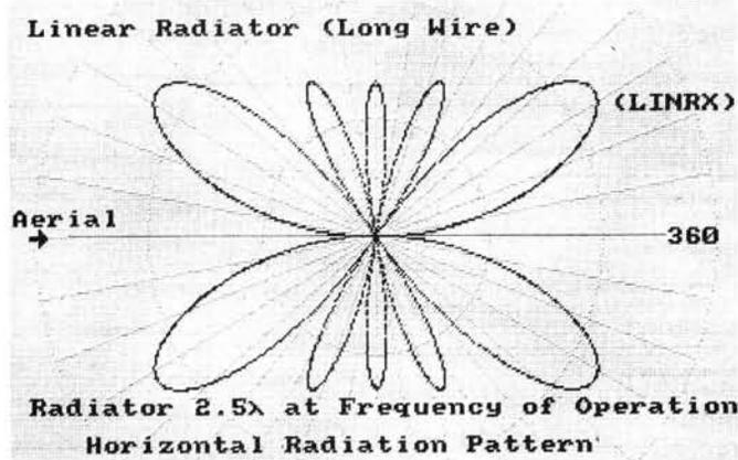
Fig. 4.3: Radiation pattern: Linear radiator 2.5 wavelengths long. Note increase in number of minor lobes
