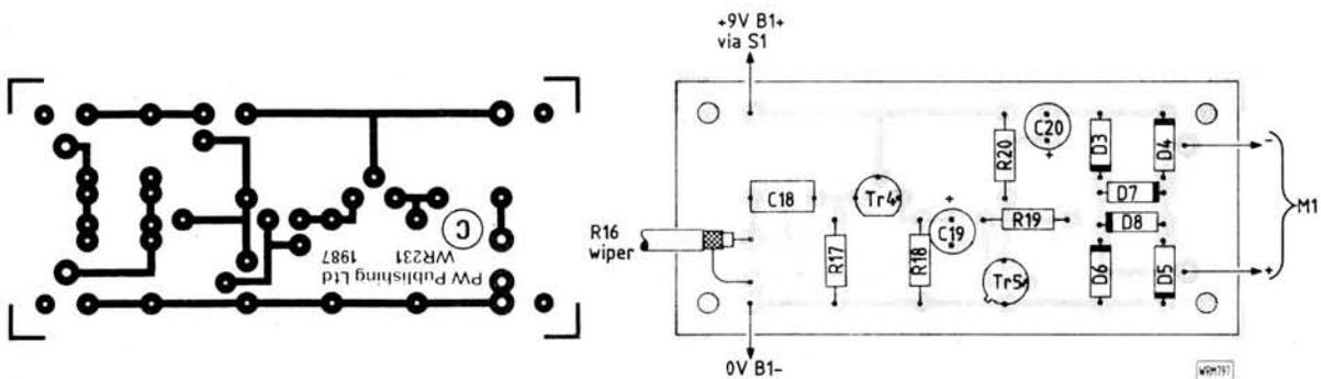
Fig. 5: Full size track pattern and component layout for indicator p.c.b.
