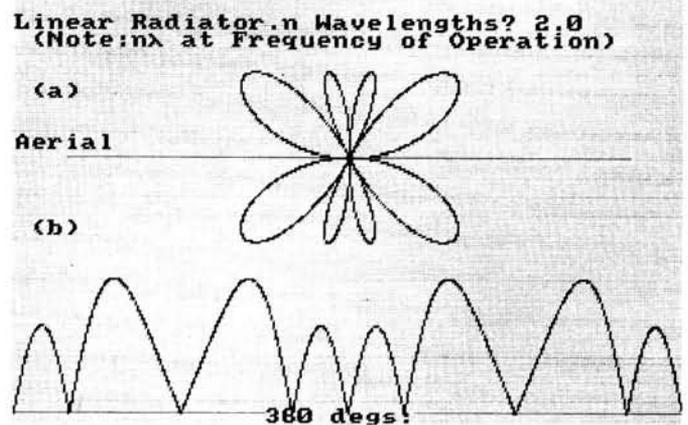
Fig. 4.2: (a) Polar pattern. Radiation at fundamental frequency of a linear radiator 2 wavelengths long. (b) For same radiator but as a Cartesian plot. (Horizontal mode)
