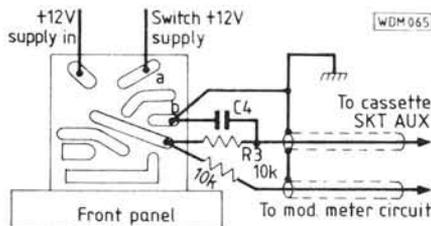
**Fig. 4: Connections to volume control p.c.b.**
