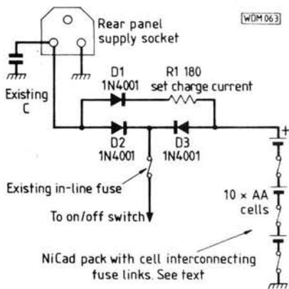
**Fig. 2: Battery pack and charger wiring showing NiCad fuse link system. (See text)**
