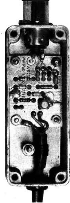
Internal view of probe. Note external ground lead connected to p.c.b.
