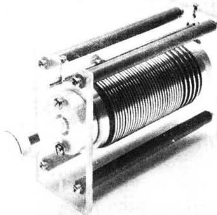
onto a special r.f.-transparent Tufnol former and has an inductance of 1 to 27 $\mu$ H. The complete roller coaster will handle up to 1kW of r.f. power without flash-over or overheating.
