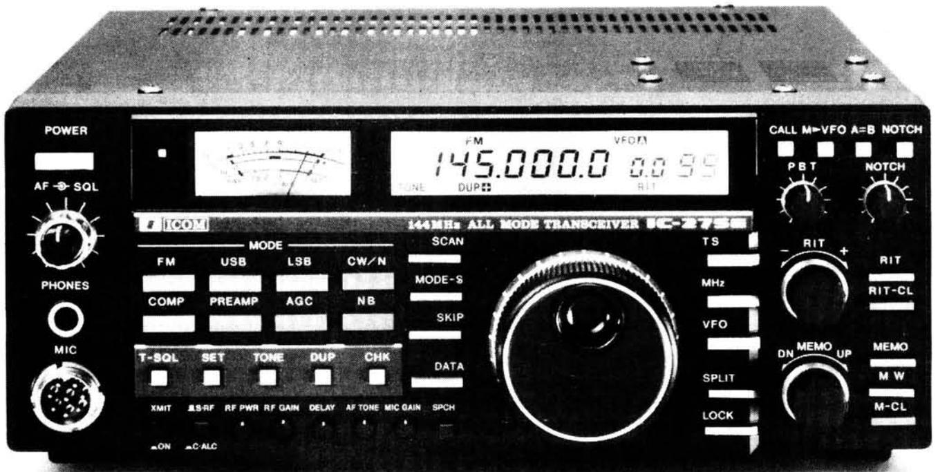
The ICOM IC-275E is the most advanced all-mode transceiver available to the Amateur today. It features a new technological breakthrough in frequency synthesizer systems. This Direct Digital Synthesizer (DDS) operates in just 5 milliseconds, providing one of the fastest transceiver lock-up times available. Ideal for PACKET and AMTOR communication modes. The IC-275E has high sensitivity and dynamic range making it an ideal unit for contests and DX operation.
