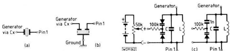
Fig. 7: Component connection points used for resonance testing
