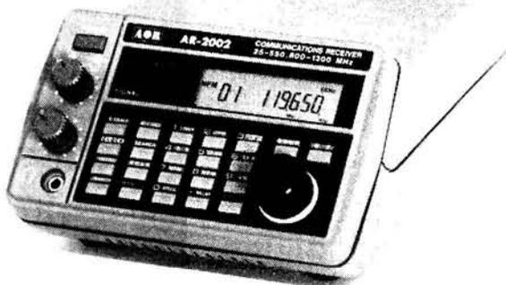
**Frequency range of the AR2002** is from 25 to 550 and from 800 to 1300 MHz. Modes of operation are wide band FM, narrow band FM and AM. The receiver has 20 memories, memory scan and a search mode which checks frequencies between user designated limits.
