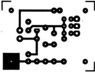
Fig. 3: Full size double sided track pattern and component layout for probe p.c.b.
