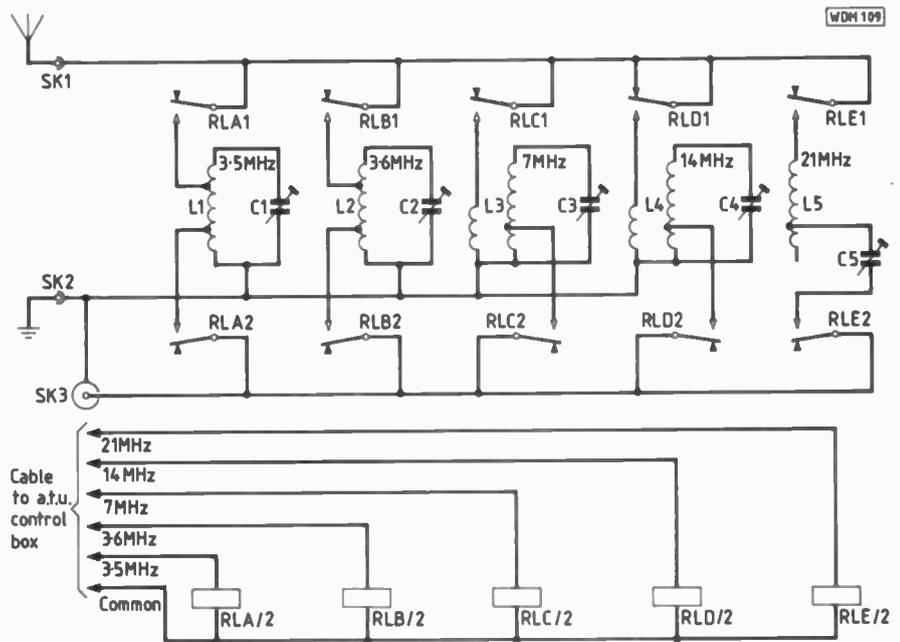
Fig. 2: Circuit diagram of remote antenna tuning unit
