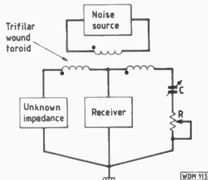
**Fig. 6: Theoretical diagram of the noise bridge.**
