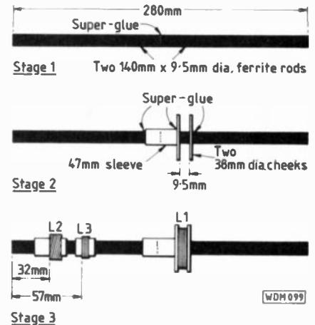
Fig. 3: Rod and coil assembly
