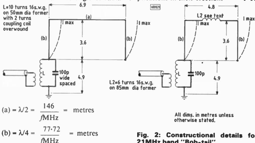
Fig. 2: Constructional details for 21MHz band "Bob-tail"
