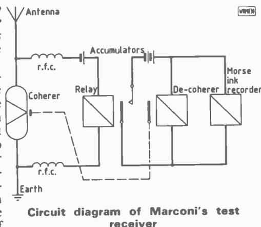
Circuit diagram of Marconi's test receiver
