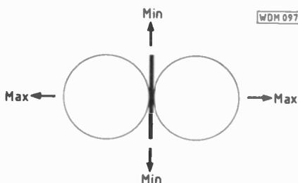
Fig. 1: Typical Polar Diagram of Ferrite Rod Antenna
