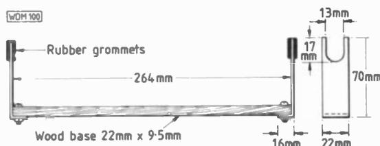
Fig. 4: Rod support frame showing bracket dimensions
