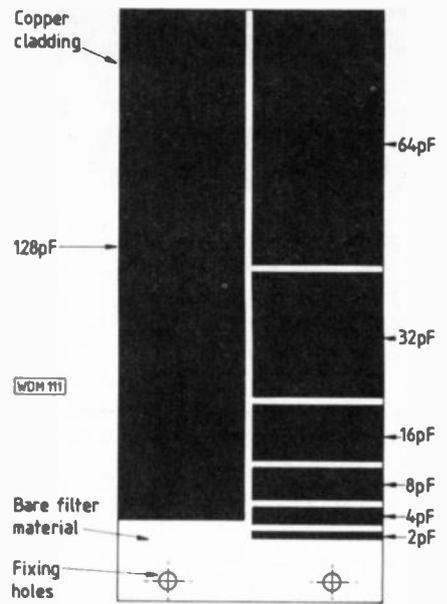
Fig. 4: Suggested layout of laminated p.c.b. capacitors
