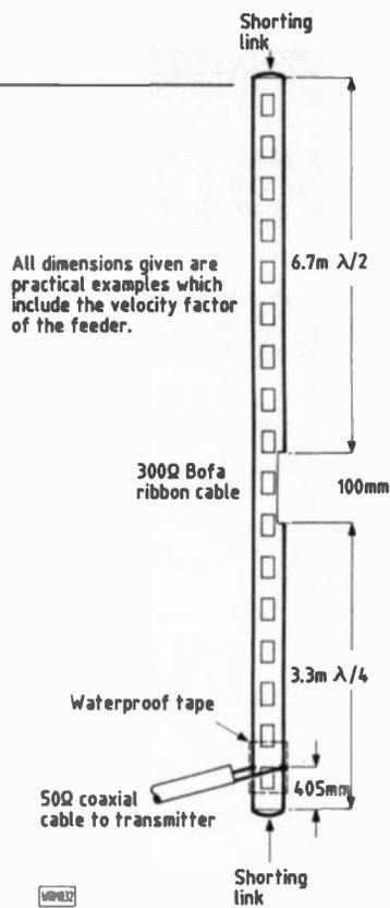
Fig. 3: "J-match" vertical for 21MHz band. Antenna can be supported in the same manner as  $5\lambda/8$  antenna
