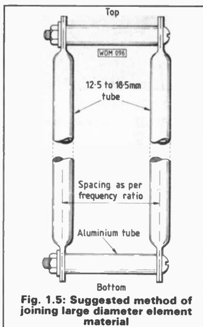
**Fig. 1.5: Suggested method of joining large diameter element material**
