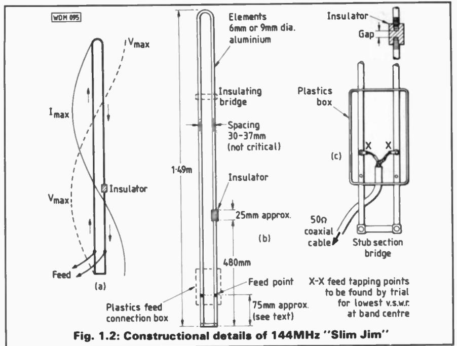
Fig. 1.2: Constructional details of 144MHz "Slim Jim"
