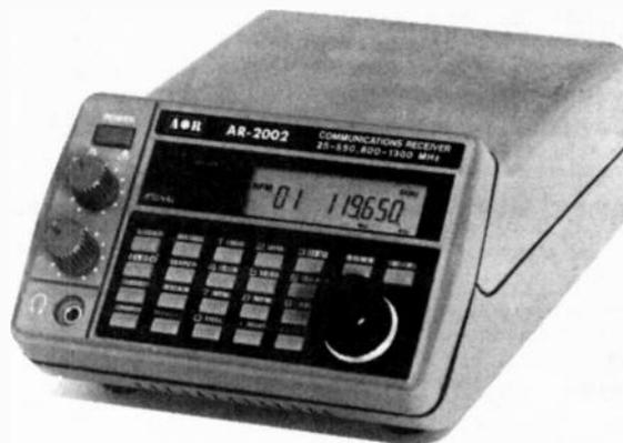
**Frequency range of the AR2002** is from 25 to 850 and from 800 to 1300 MHz. Modes of operation are wide band FM, narrow band FM and AM. The receiver has 20 memories, memory scan and a search mode which checks frequencies between user designated limits.
