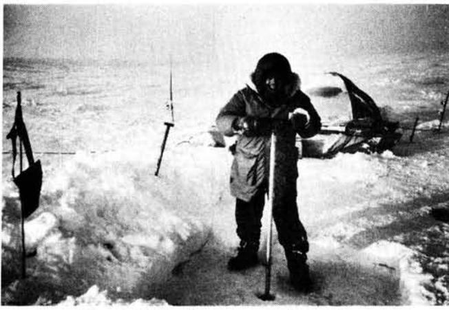
**Hand-drilling ice-cores to 10m takes two days at  $-45^{\circ}\text{C}$ , east of Ward Hunt Island**
