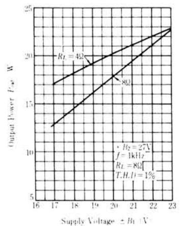
**Fig. 4: Output power vs supply voltage**
