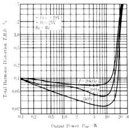
**Fig. 3: Total harmonic distortion vs output power**
