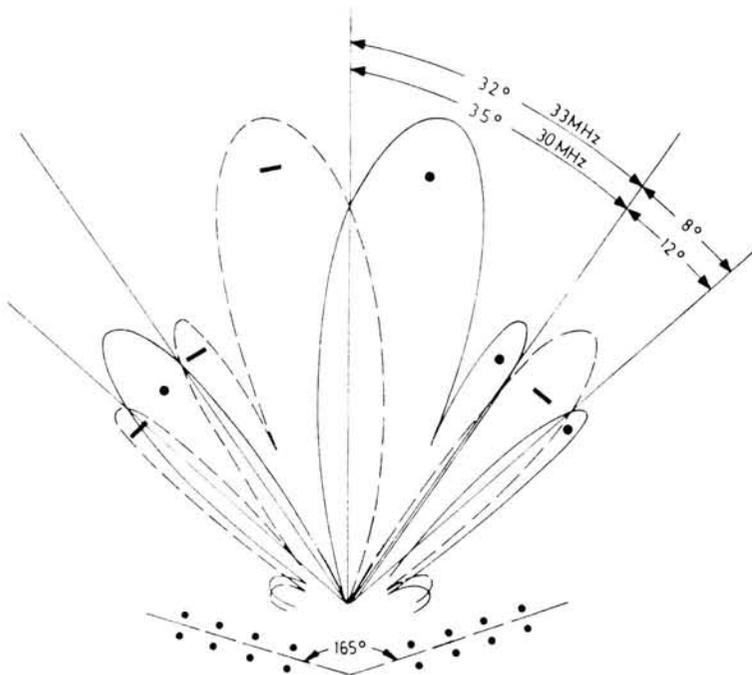
Fig. 1.6: The antenna pattern of the Knickebein array
