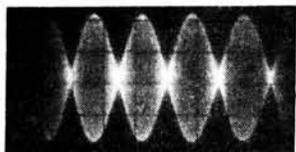
Two waveforms showing a typical modulation envelope
