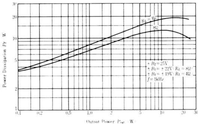
**Fig. 5: Power dissipation vs output power**
