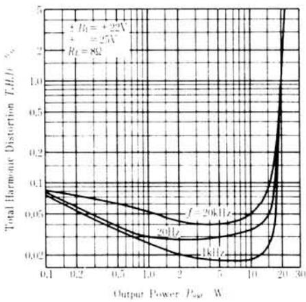
**Fig. 2: Total harmonic distortion vs output power**
