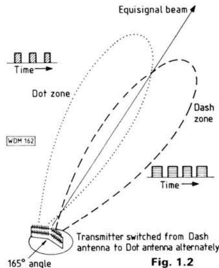
Fig. 1.2: The principle of the Lorenz (Knickebein) beam
