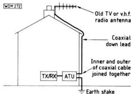
Fig. 2.3: The "phoney" TV antenna that can get around local regulations
