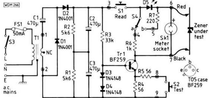
Fig. 1: Circuit diagram of Zener tester
