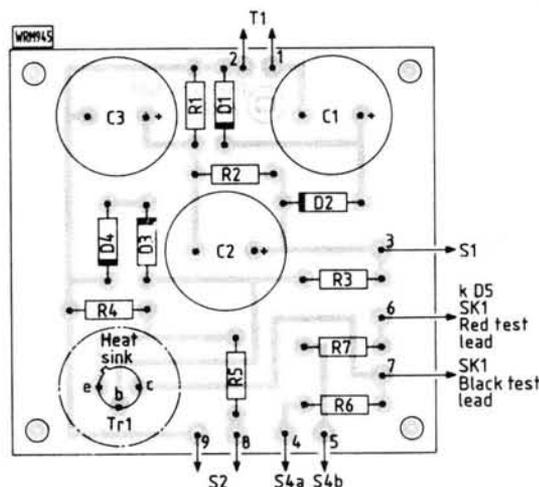
**Fig. 3: Full size p.c.b. track pattern and component placement diagram**
