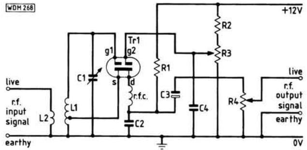
Fig. 6.3: A regenerative detector using a dual-gate m.o.s.f.e.t.
