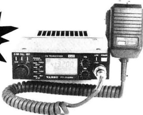
We are pleased to announce a new series of FM VHF and UHF mobile transceivers for the amateur. The 45/5W FT-212RH and the 35/4W FT-712RH. Smaller than their predecessors these models utilize a new cpu with greatly expanded features, most notable of which are 19 memories and support for the DVS-1 Digital Voice System, which can digitally record and playback from the microphone or the receiver.
