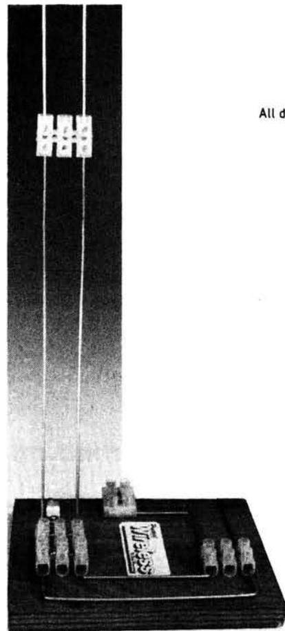
bottom of the radiating element. The positions of the blocks may require shifting slightly to obtain a symmetrical layout. After this has been achieved they may be screwed into place.
