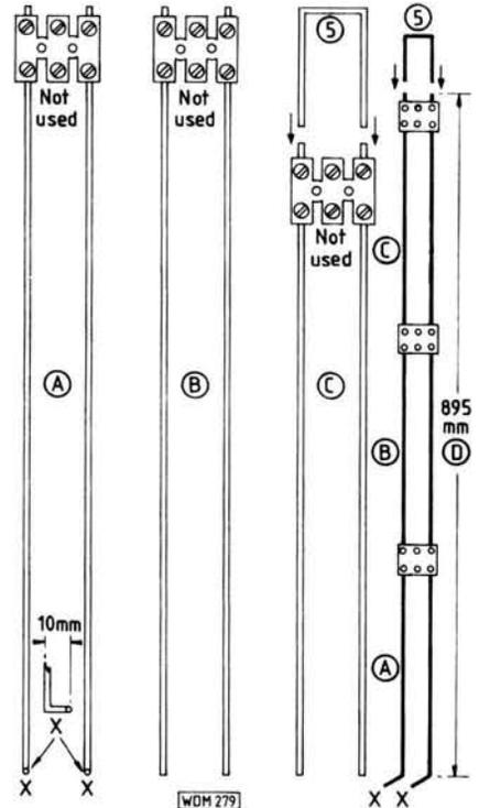
**Fig. 5: The radiating element consists of sections A, B and C. Together they form the vertical radiator, with an overall dimension of 895mm. Note including section No. 5. Also note right angle bends at the bottom of section A. These connect to points (X, X) on the base board as in Fig. 3.**
