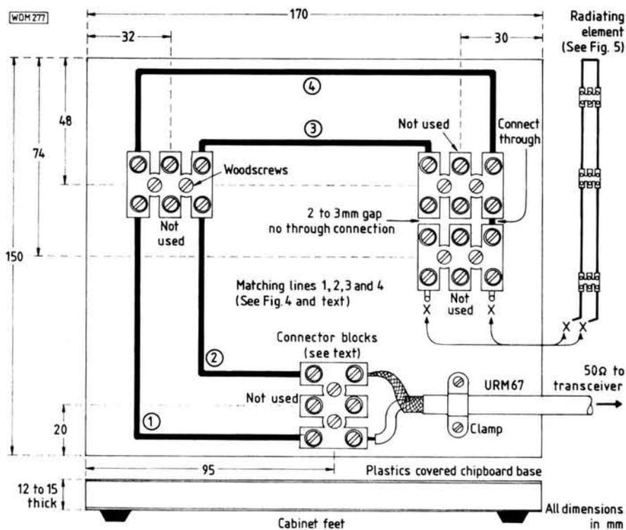
**Fig. 3: Layout on baseboard of the matching lines which are comprised of (1 and 4) and (2 and 3) sections. Note the bottom of radiator element wires are secured at (X, X)**
