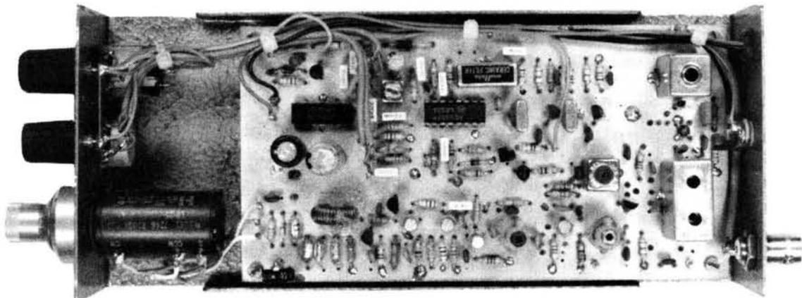
Internal view of prototype receiver
