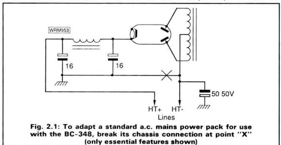
**Fig. 2.1:** To adapt a standard a.c. mains power pack for use with the BC-348, break its chassis connection at point "X" (only essential features shown)
