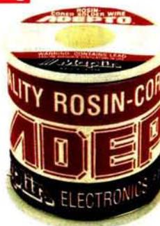
Top quality standard flux-cored solder designed for hand and machine soldering of electronic components. Manufactured to BS219 Grade KP, BS441 Grade 2 and BS5625 Class 5a. The solder is a 60% tin, 40% lead alloy containing a non-corrosive flux. Solder starts to melt at 183°C and is fully molten at 188°C. Available on 1/2kg reels in 0.7mm dia. (22 swg) and 1.2mm dia. (18 swg). Perfect for use with all hand soldering irons including Antex, Weller etc.
