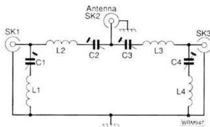
Fig. 1: Circuit diagram of the 144MHz/430MHz diplexer
