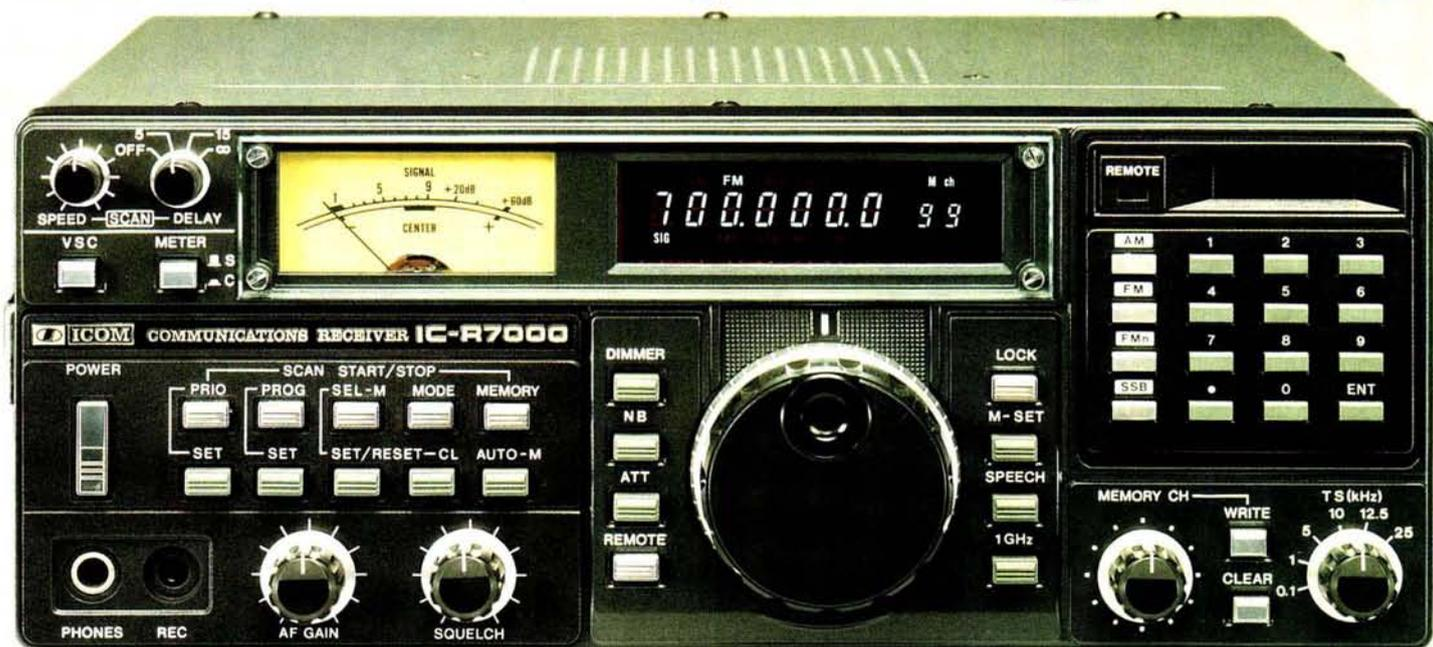
With 99 programmable memories the IC-R7000 covers aircraft, Marine, FM Broadcast, Amateur Radio, television and weather satellite bands. For simplified operation and quick tuning the IC-R7000 features direct keyboard entry. Precise frequencies can be selected by pushing the digit keys in sequence of the frequency or by turning the main tuning knob. FM wide/FM narrow/AM upper and lower SSB modes with six tuning speeds: 0.1, 1.0, 5, 10, 12.5, 25KHz.
