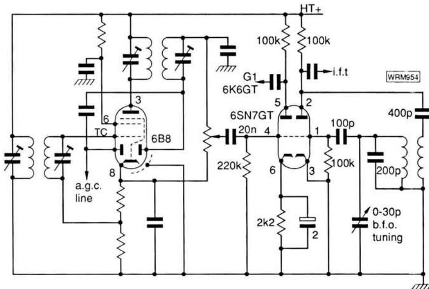
**Fig. 2.2: Modifications to the last i.f./b.f.o. stages (-J and later marks) to include an extra a.f. amplifier, plus a continuously variable-tuned b.f.o. for s.s.b. reception. New components have values shown; existing components do not. The b.f.o. coil is the redundant i.f./xtal coupler removed from set (see text)**
