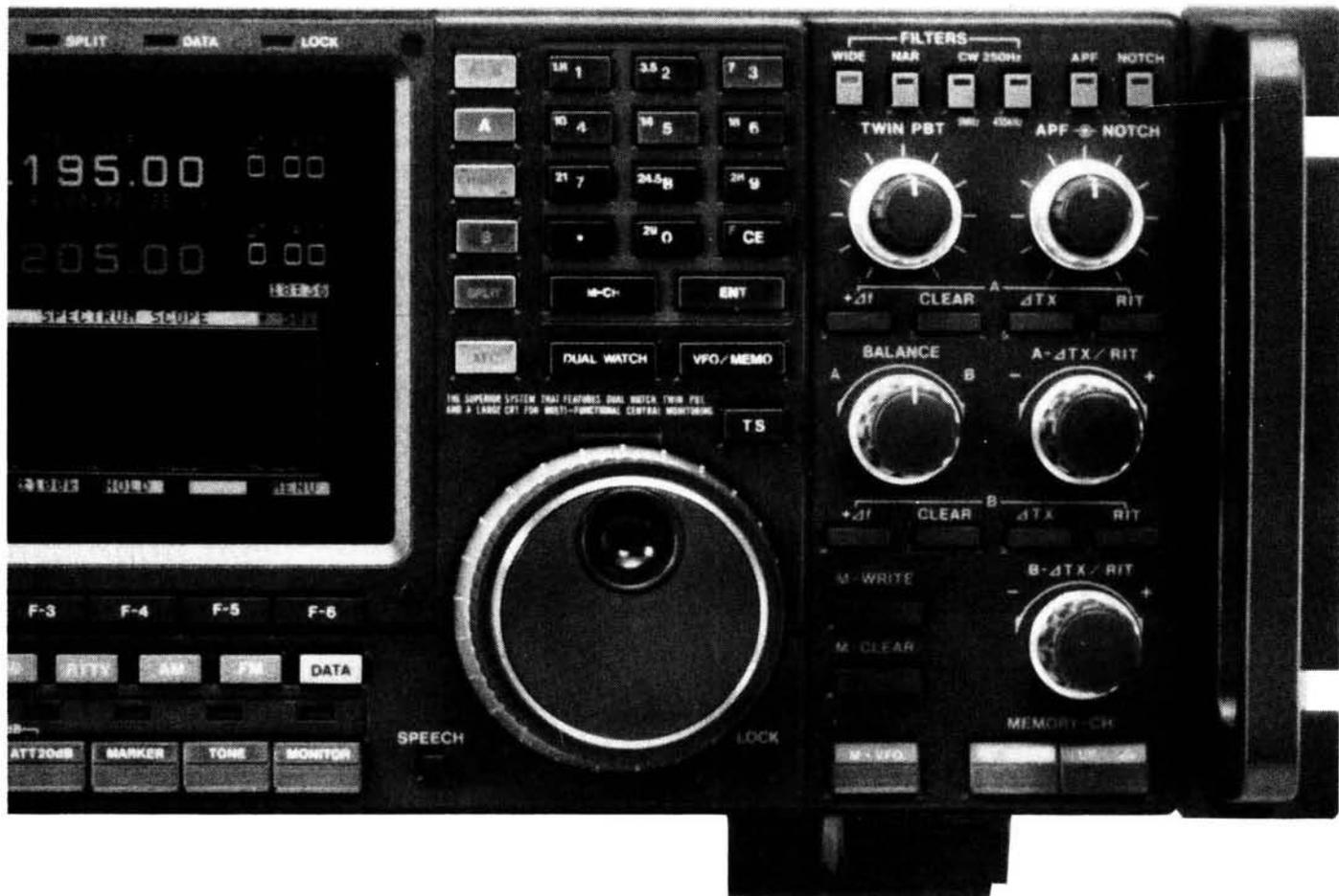
The IC-781 has a dual-watch function which allows simultaneous receive of two frequencies in the same band. Balance controls adjust VFO A/B receive strength levels. This feature is especially useful on Dx-expeditions or contests to check band activity or to tune in your next contact. The newly developed ICOM DDS (Direct Signal Synthesizer) system is incorporated to provide a fast transceiver lock-up time. This is essential for data communication systems.
