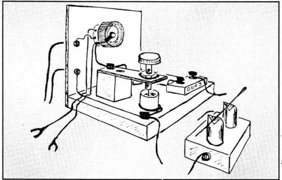
Fig. 4.2: Sketches of replicas of the Fessenden detector and the Massie Oscillaphone
