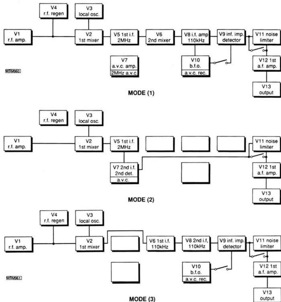
**Fig. 1.1: The circuit arrangements for each of the three modes of operation, simplified to block diagram form**
