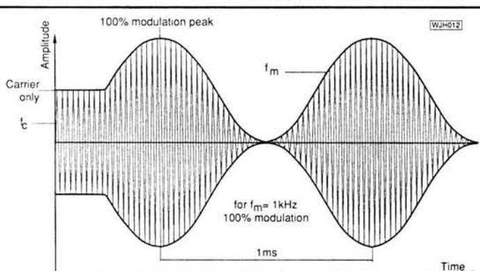
Fig. 9.2: Amplitude modulation as seen on an oscilloscope
