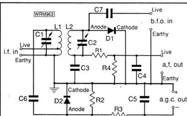
Fig. 9.1: An envelope detector for a.m. signals with a.g.c. rectification
