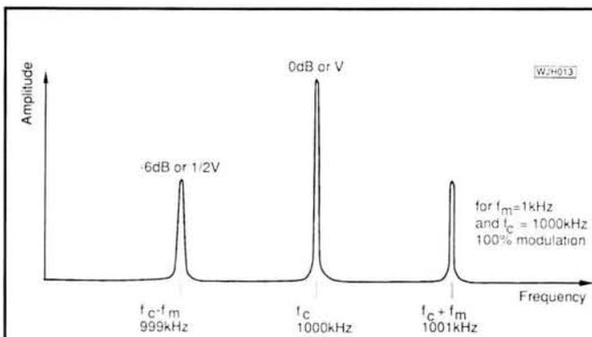
**Fig. 9.3: Amplitude modulation as seen on a spectrum analyser**
