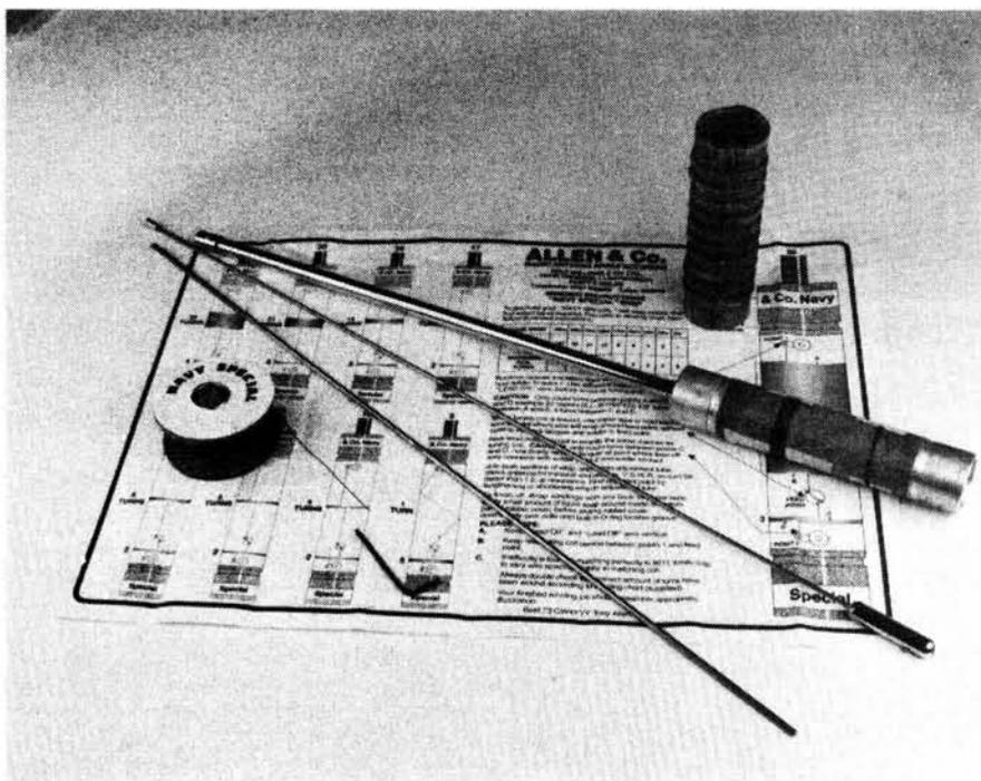
*Paul Essery GW3KFE has been trying out an unusual design of mobile antenna. The "Navy Special" can be wound by the user to suit any one of the h.f. amateur bands from 3.5MHz upwards, or the 144MHz v.h.f. band. Tuning around any chosen band is achieved by adjusting the length of the whip for a precise match to the chosen frequency.*
