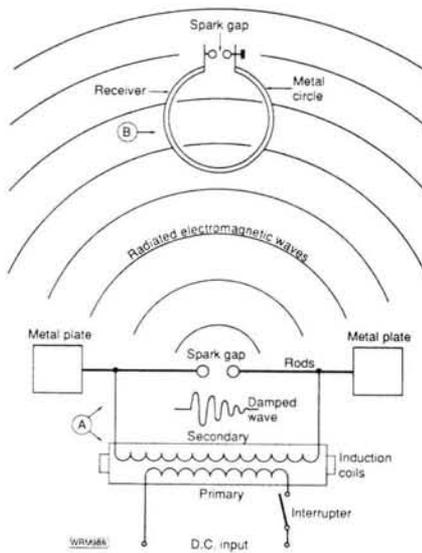
**Fig. 1: (a) The induction coil and capacity radiator used by Hertz to generate electromagnetic waves. (The "transmitter" and Hertzian dipole). (b) The ring resonator "receiver" used for the detection of electromagnetic waves at a distance from the "transmitter"**
