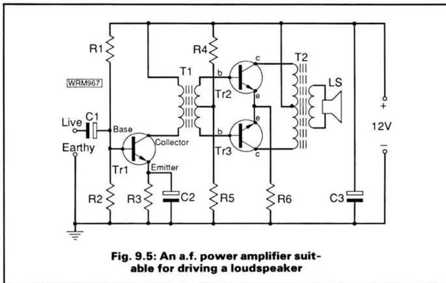
Fig. 9.5: An a.f. power amplifier suitable for driving a loudspeaker
