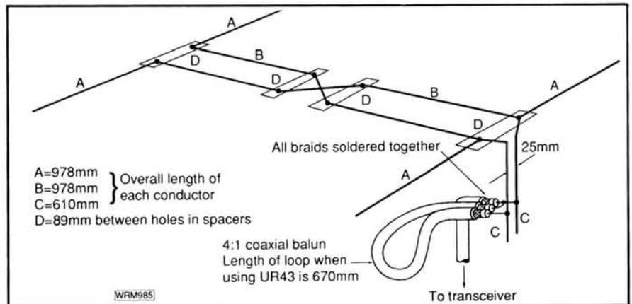
**Fig. 1: Main antenna elements are made from pvc insulated conductors stripped from either 1.00mm<sup>2</sup> or 2.5mm<sup>2</sup> twin and earth mains cable**
