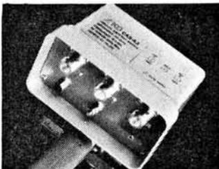
ALLOWS SELECTION OF 2 ANTENNAS FROM 1 COAX FEEDER
