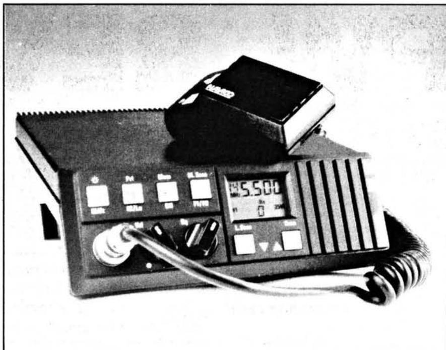
when you press the p.t.t., there is a carrier present, the tone burst is disabled, if however there was no carrier present, the tone burst circuit sends out a 400ms burst of 1750Hz to access the repeater. The idea is so simple I can't imagine why everyone isn't doing it, so full marks to Navico for some smart thinking!
