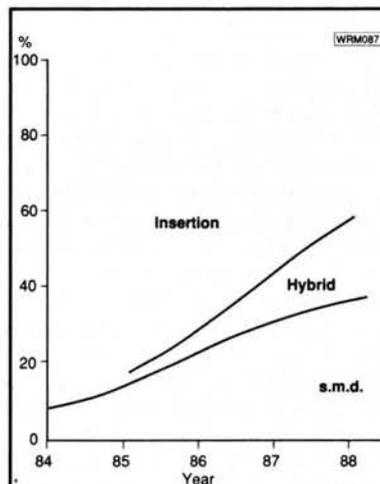
Fig. 1.1: Increasing usage of s.m.d.s in circuit fabrication
