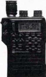
The Standard C150 super-compact 2m transceiver having all the usual features that you would expect from a modern microprocessor controlled radio — plus several new ones. Extendable frequency range on RX.
