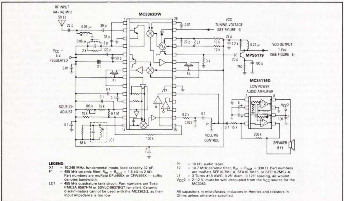
Fig. 4: Synthesised 144MHz f.m. receiver
