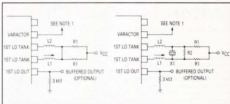
**Fig. 2: Alignment circuit for first local oscillator**
