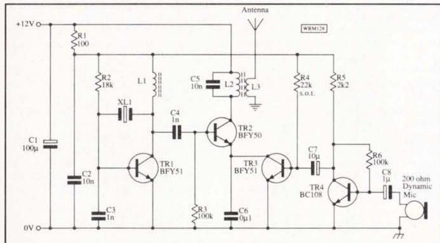
Fig. 1: Circuit diagram of the experimental transmitter
