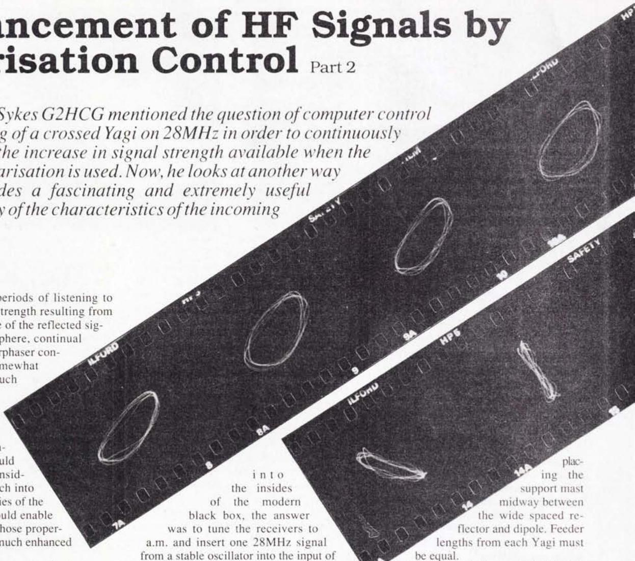
into the insides of the modern black box, the answer was to tune the receivers to a.m. and insert one 28MHz signal from a stable oscillator into the input of each receiver thus producing an in-phase b.f.o. on each.
