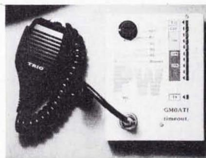
the microphone transmit switch is released or after IC1 has counted and decoded clock inputs until the final l.e.d. is illuminated. At which point gate IC2d changes state switching off TR1 allowing RL1 to drop out and the rig returns to receive.
