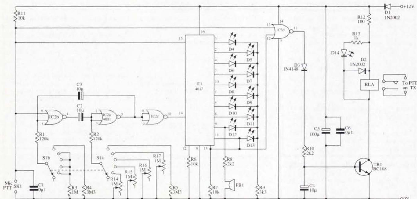
Caution should be exercised when handling the c.m.o.s. devices as they are easily damaged by high levels of static built up in a body wearing Nylon clothing, or walking on carpets made of synthetic material. This static build up may be discharged before handling these devices, by touching an earthed object such as a radiator or water tap.
