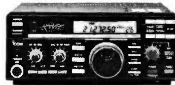
Compact HF transceiver with General coverage receiver. 26 memories, 100 watts output. All band, all mode, (FM optional).
