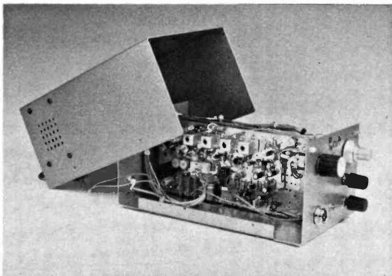
Check every other component for placing and orientation on the board and then finally solder the crystal or crystals into position with the minimum of heat and physical strain. Once again check for dry joints and or solder bridges. A check for shorts between the supply lines with an Ohmmeter completes the construction
