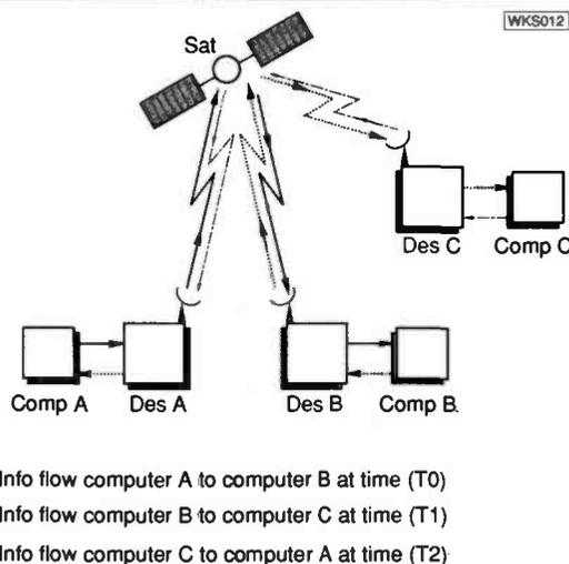
**Fig. 2: Multiple access techniques increase efficiency and availability**
