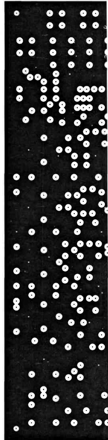
WRM244    Ⓢ Holes marked thus are pins which must be soldered both sides of board
