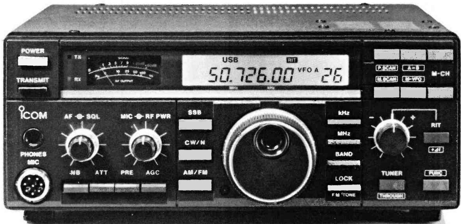
The new ICOM IC-726 is a compact, easy to use transceiver which covers the amateur bands from 1.8 to 50MHz. It can be used in your home, car and in portable locations on SSB, CW, AM and FM modes.
