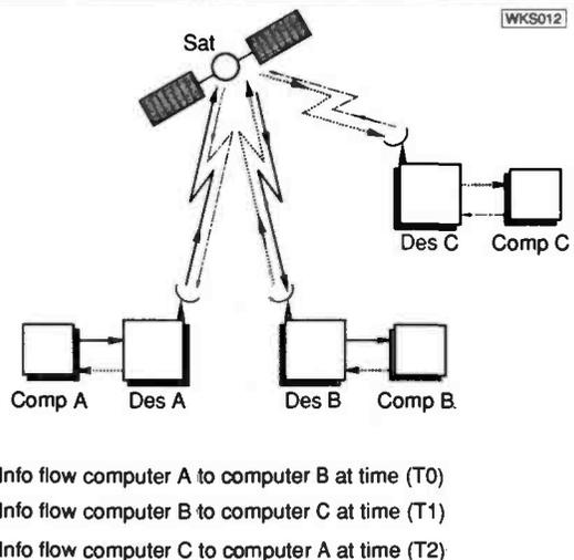
**Fig. 2: Multiple access techniques increase efficiency and availability**
