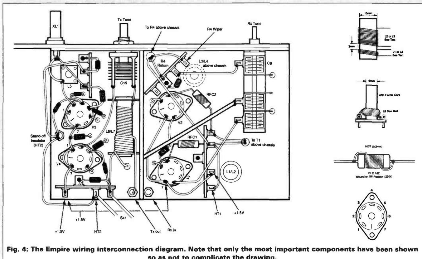
Fig. 4: The Empire wiring interconnection diagram. Note that only the most important components have been shown so as not to complicate the drawing.
