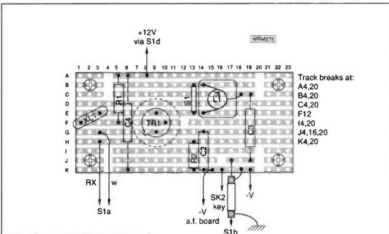
Fig. 2.1a: Oscillator board.
