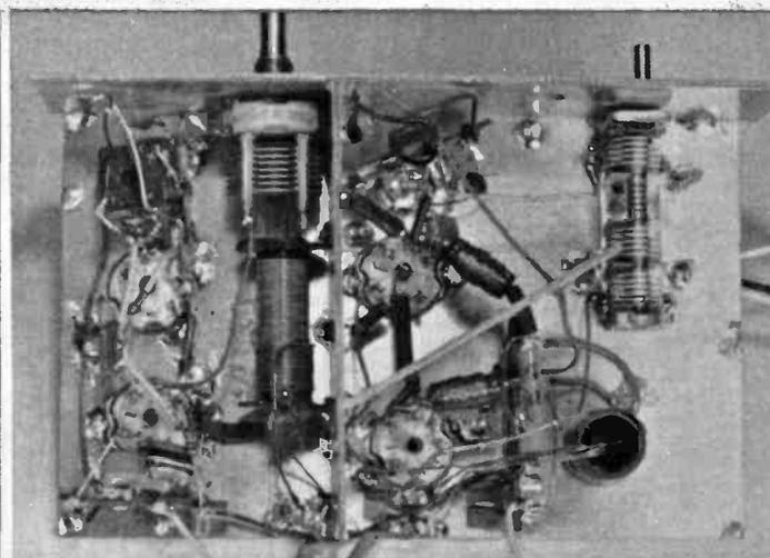
Under-chassis view showing L6/7 and main receiver tuning capacitor in position.
