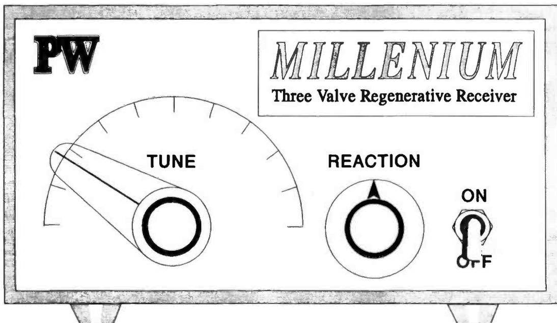
*The front panel overlay for the PW Millennium Regenerative Receiver (not to scale)*
