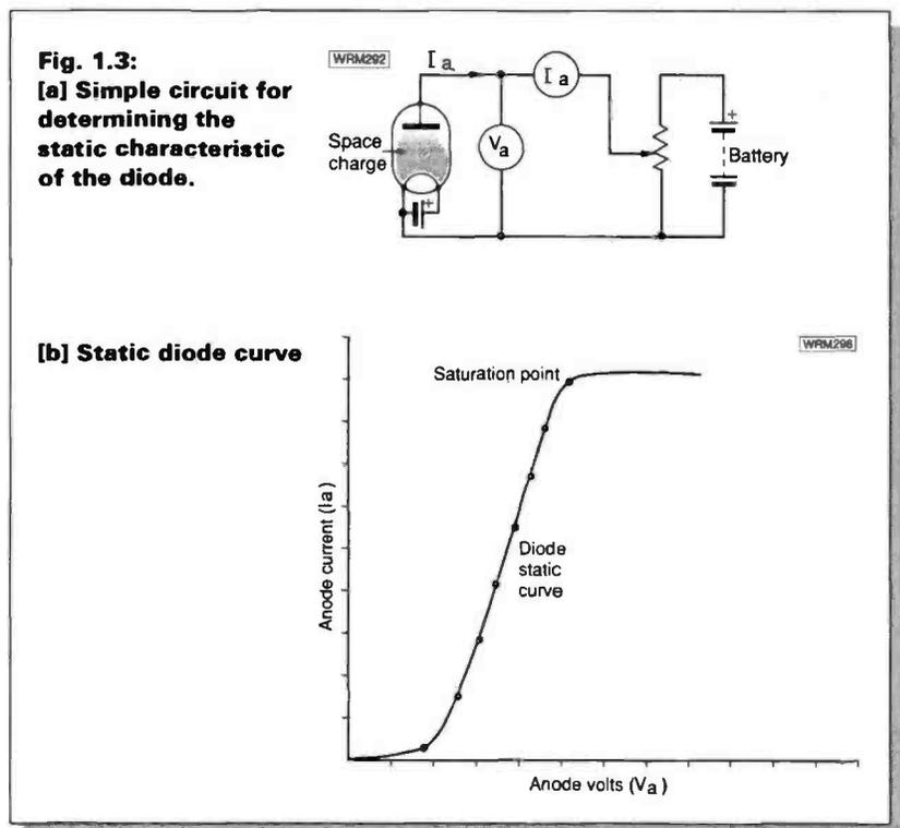
**Fig. 1.3: [a] Simple circuit for determining the static characteristic of the diode.**
