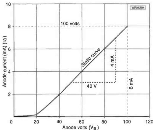
**[b] Static with load showing diode operating point.**
