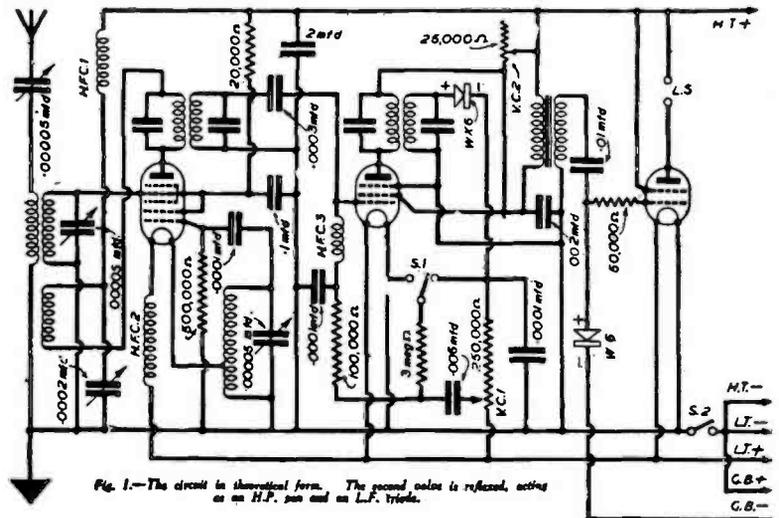
Fig. 1.—The circuit in theoretical form. The second coil is reflexed, acting as an H.F. coil and an L.F. triode.
