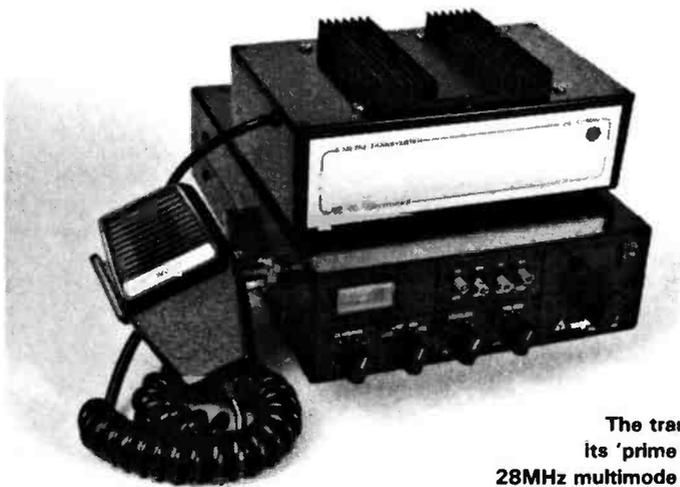
The transverter and its 'prime mover' — a 28MHz multimode transceiver.
