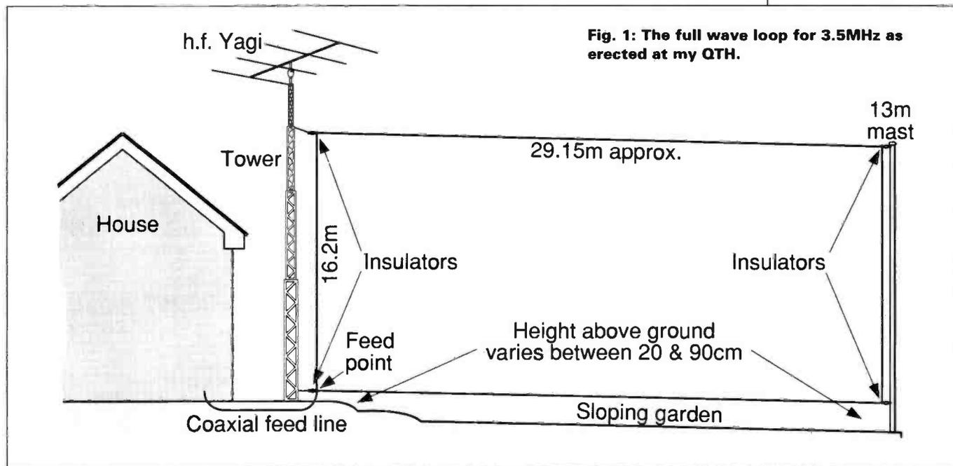
Fig. 1: The full wave loop for 3.5MHz as erected at my QTH.
