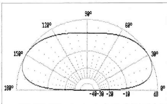
**Fig. 3: Radiation pattern of the full wave loop with the feed point half way down one side. The 0dB reference curve is 4.98dBd at 3.510MHz.**
