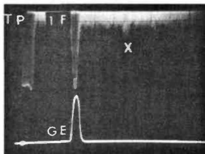
**Fig. 14. Oscillogram. (S) Echo from ionosphere (F region). with splitting due to the earth's magnetic field. (magneto-ionic splitting). (G) Superimposed gating-pulse, opened-out so that the whole of echo and some receiver noise is displayed.**
