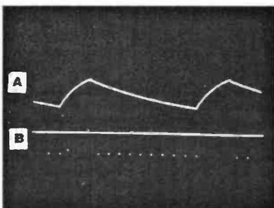
Fig. 11. Oscilloscope. (A) Timebase wave. (B) Very short duration ( $0.5\mu\text{s}$ ) marker pips. (See text regarding a specific application).
