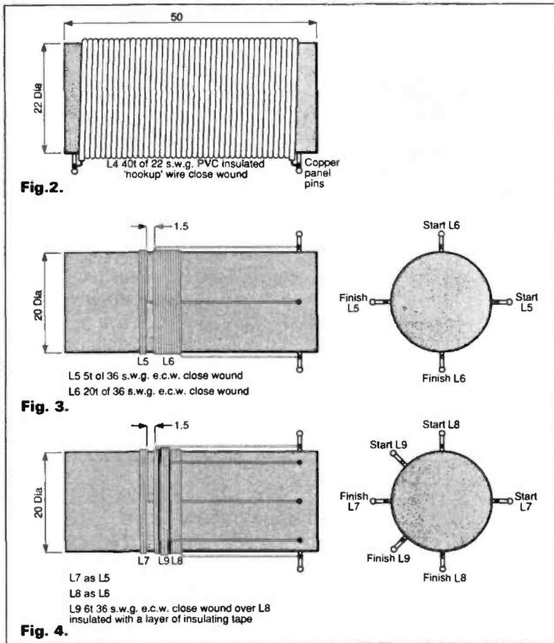
**Fig. 2:** This coil (L4) wound on a piece of wooden dowelling) is for the  $\pi$ -matching unit.
