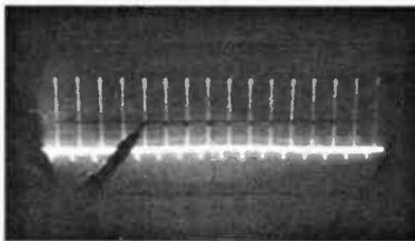
Fig. 8. Oscilloscope. Method of calibrating a timebase with narrow marker pulses of known frequency. Example pulse intervals =  $10\mu\text{s}$ . (see also Fig. 9 and text).
