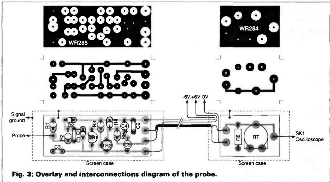
**Fig. 3: Overlay and interconnections diagram of the probe.**
