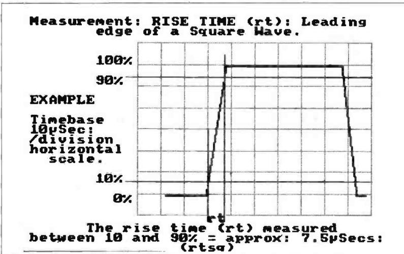
**Fig. 5. The 'rise-time' of a squarewave is measured over 80% of the leading edge i.e., between 10 and 90%.**
