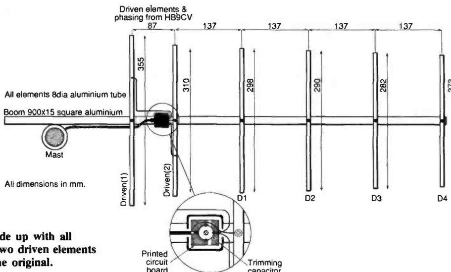
**Fig. 2:** This is how the antenna is made up with all dimensions of the new elements. The two driven elements from the HB9CV antenna are as in the original.
