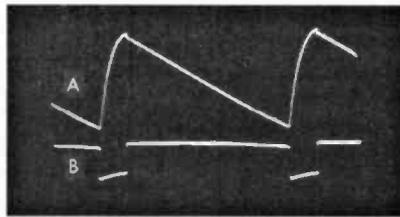
Fig. 7. Oscilloscope. (A) Miller-transition timebase with (B) initiating . Commonly used with older 'valved' scopes.
