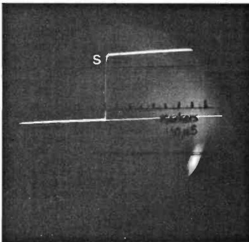
Fig.9. Oscilloscope.  $10\mu\text{s}$  markers inked onto uncalibrated graticule. Rise-time of square wave (S) also displayed, is virtually  $1\mu\text{s}$ .
