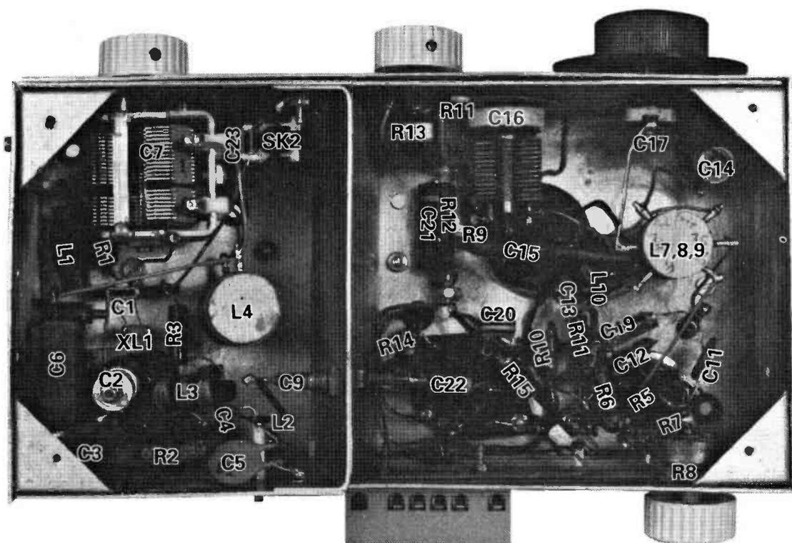
Fig. 6: Layout of the underside, showing the plate dividing the transmitter from the receiver.
