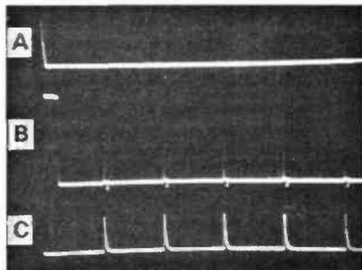
**Fig. 13. Oscillogram. (TP) Transmitted r.f. pulse (50µs). (1F) Echo from the ionospheric F region. (GE) Same echo but gated to eliminate noise etc. (X) A secondary echo (2F) just above the receiver noise. See text for further explanation.**
