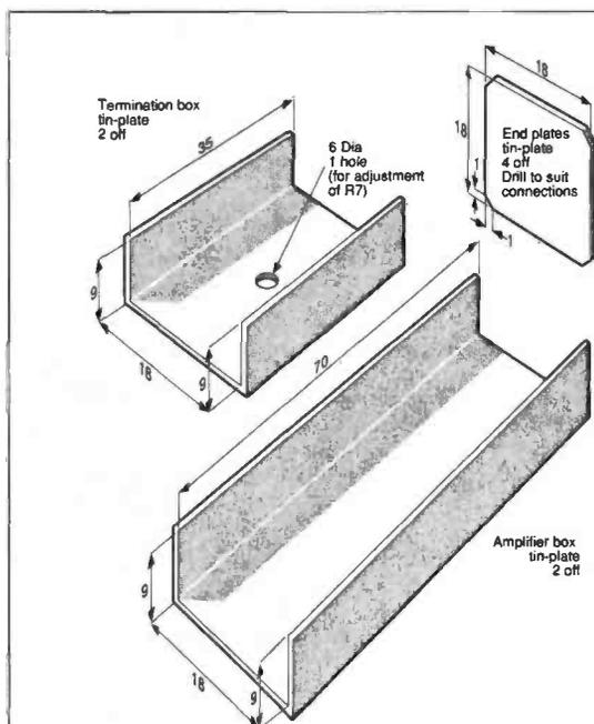
**Fig. 4: Basic measurements of the three shapes required to make the probe screening boxes.**
