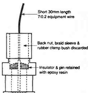
**Fig. 5: One idea for a possible interchangeable probe tip.**
