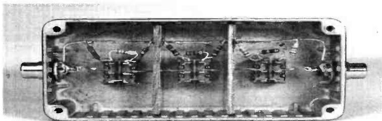
**Fig. 4a. A view of the attenuator mounted in its box.**
