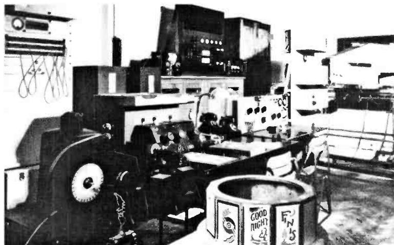
**Fig. 4: The BBC television control room at 16 Portland Place in London in 1935. Caption machine in foreground, with disc scanner on the left, with twin monitor receivers above. The mirror-drum scanner (the camera) is pointing into the studio.**
