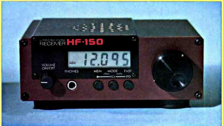
**Aerial inputs:** 600 ohms, 50 ohms & Hi-Z Whip
