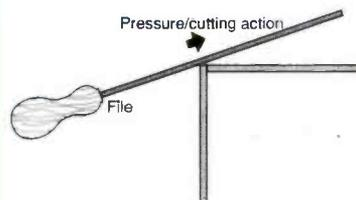
**Fig. 6:** Using a file to finish the edges of a box.
