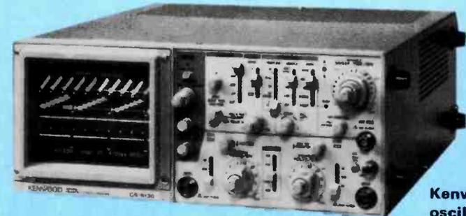
**Kenwood 40MHz readout oscilloscope, CS-5130.**
