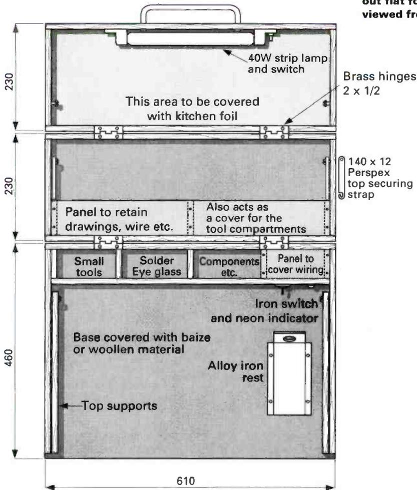
Fig. 2: The completed table-top project bench.
