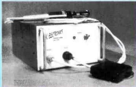
**AK Electronics de-solder station, Model R2100.**
