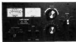
This linear is incredible value. We have put it through its paces and it really stands abuse. 3 rugged 811A tubes provide up to 600 Watts output from 160-10m. A hunky mains transformer and full metering is included. Used by DX-peditions it has to be amazing value at £699 inc VAT
