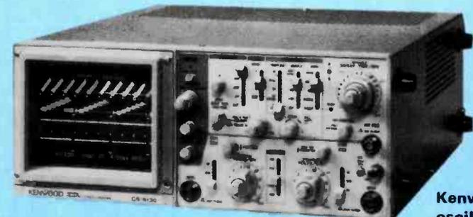
**Kenwood 40MHz readout oscilloscope, CS-5130.**
