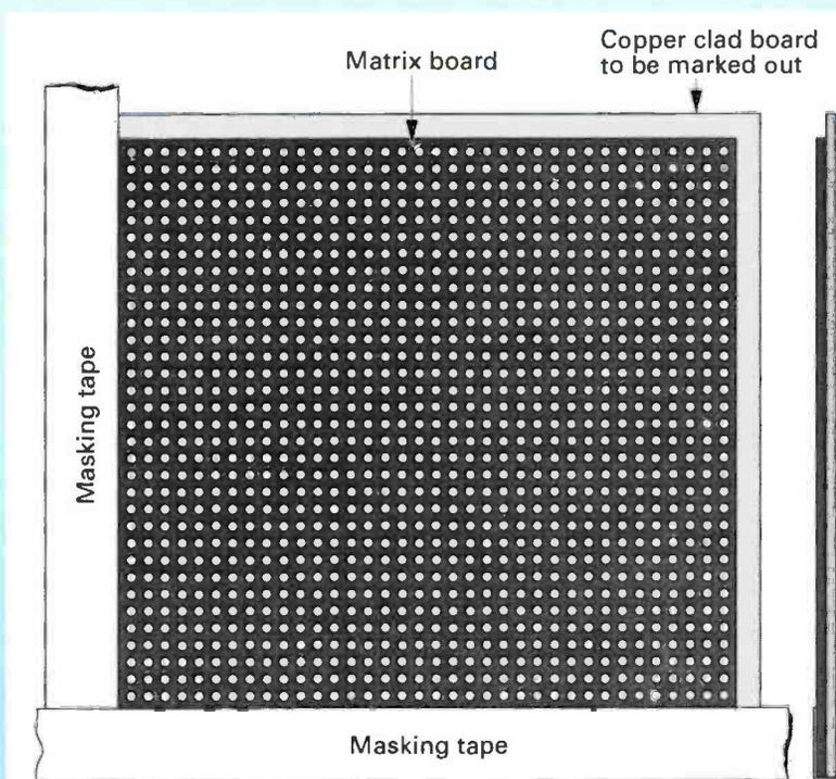
**Fig. 1: The matrix board is taped to the copper-clad board as shown here.**
