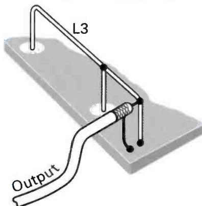
**Fig. 3: Detail for bending L1 and L3 (L3 shown here). The tapping point for L1 is above the middle connection. The tapping point on L1 is not the same as the tapping point for L3 shown here.**
