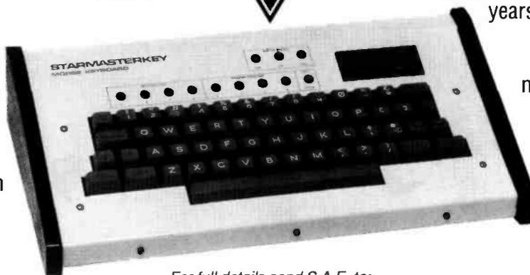
4 message memories each of 255 characters. 26 message memories each of 127 characters. All memories stored on non volatile. Ram-messages stored for up to 5 years. indication of speed on 7 segment display. Indication of operating mode on LEDs. Sidetone and relay output for all types of transmitter. Full QWERTY keyboard with real keys. Metal cased for RF immunity.
