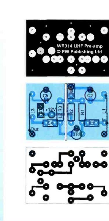
Fig. 2: The track pattern and overlay of the pre-amplifier p.c.b. See Fig. 3 for more details of L1 and L3.
