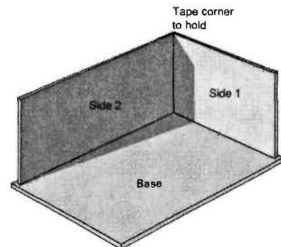
**Fig. 3:** Assembling the box, using tape to hold the corners together before the adhesive is applied.
