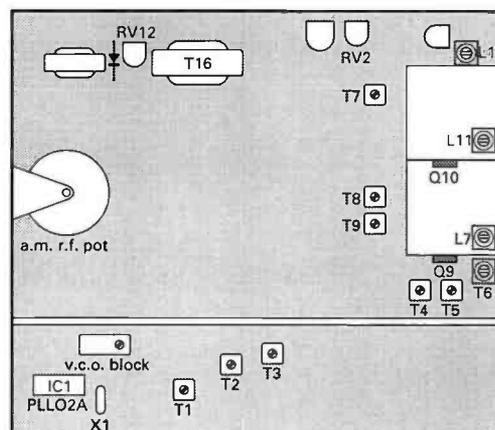
Fig. 2: Diagram showing main board lay-out on the transceiver, with main components and those involved in the conversion indicated.
