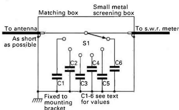
**Fig. 7: A suitable matching system for the mobile antenna. See text for method used to select the capacitors.**
