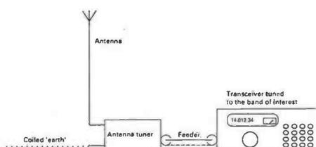
Fig. 2: An experimental layout for a helically-wound earth, with a trapping facility incorporated.
