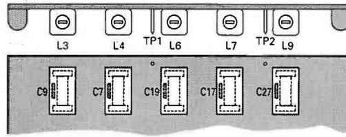
**Fig. 4: The receiver multiplier board. To carry out the modifications the screening cans have to be removed (see text).**
