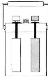
Fig. 3: The basic lay-out (simplified) of a directly-heated triode.
