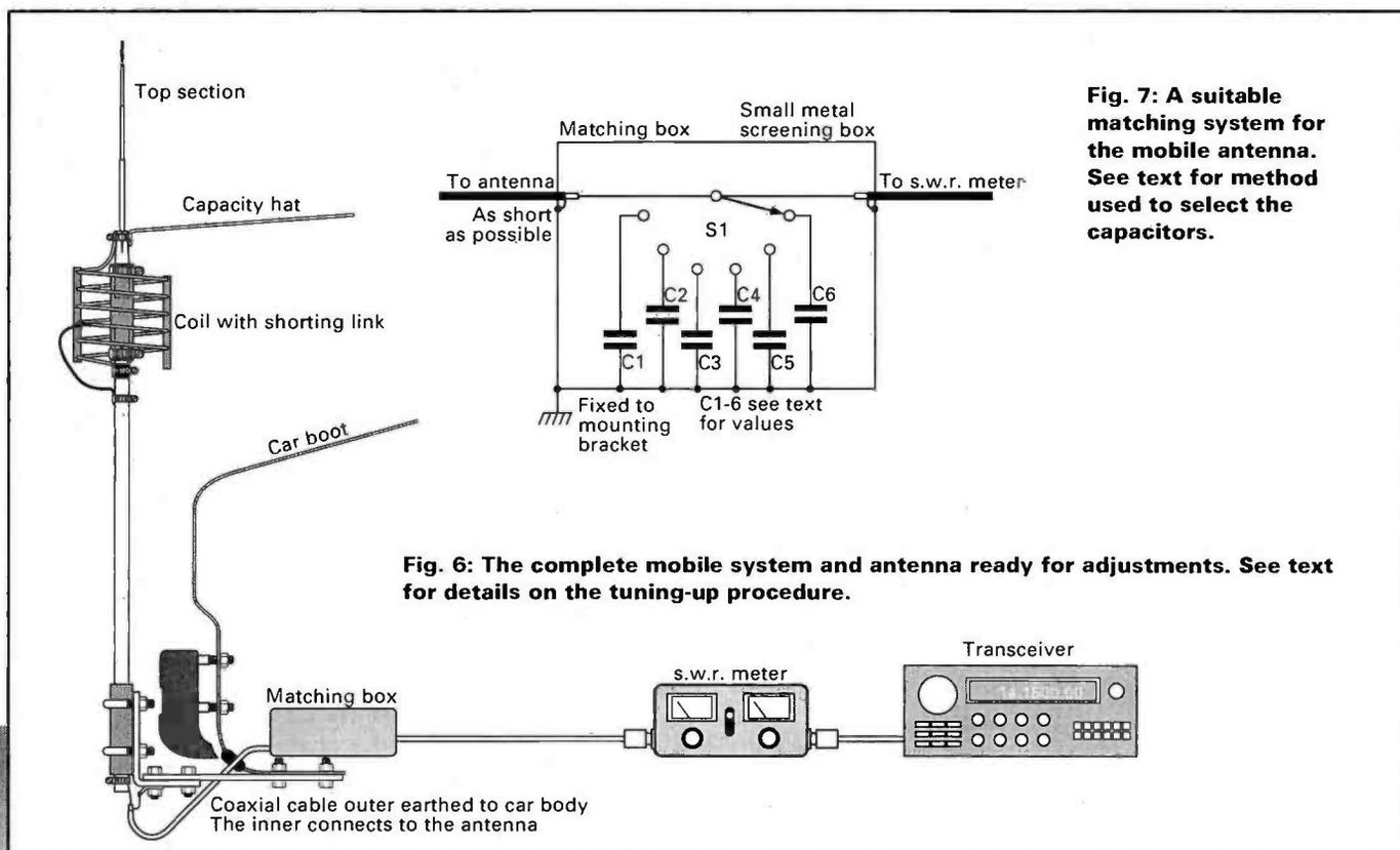
**Fig. 6: The complete mobile system and antenna ready for adjustments. See text for details on the tuning-up procedure.**
