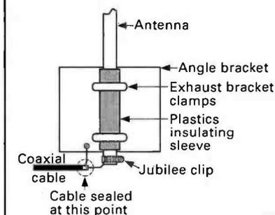
**Fig. 3: Details of angle bracket, showing use of exhaust bracket clamps. The end of the coaxial cable must be sealed and made fully waterproof.**
