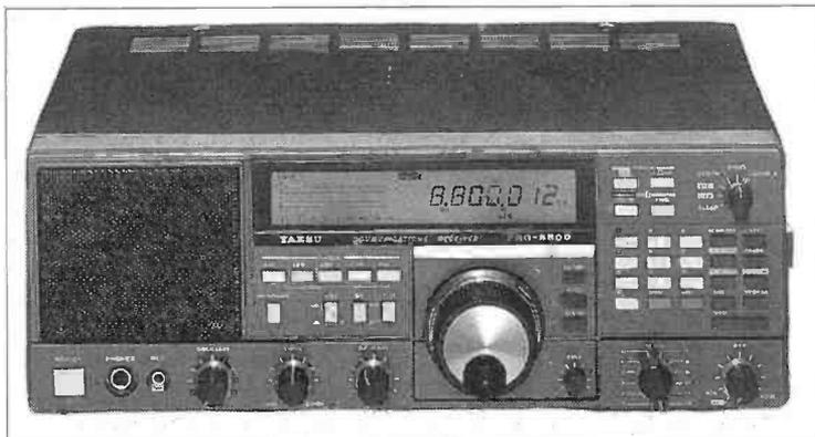
I used the BBC micro, as I had one laying around, although any computer that has the facility of a serial port that has a capability of running at 4800 bauds could be used to control the FRG-8800.
