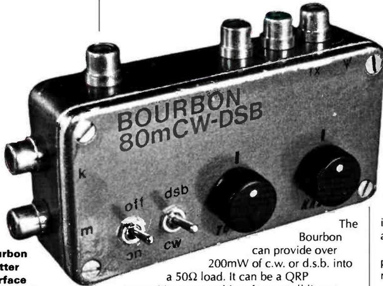
The Bourbon transmitter uses surface mount technology to pack a lot into a small space.
