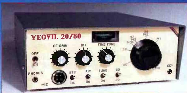
**G4SLU Builds The Yeovil 3.5 And 14MHz HF Transceiver**
