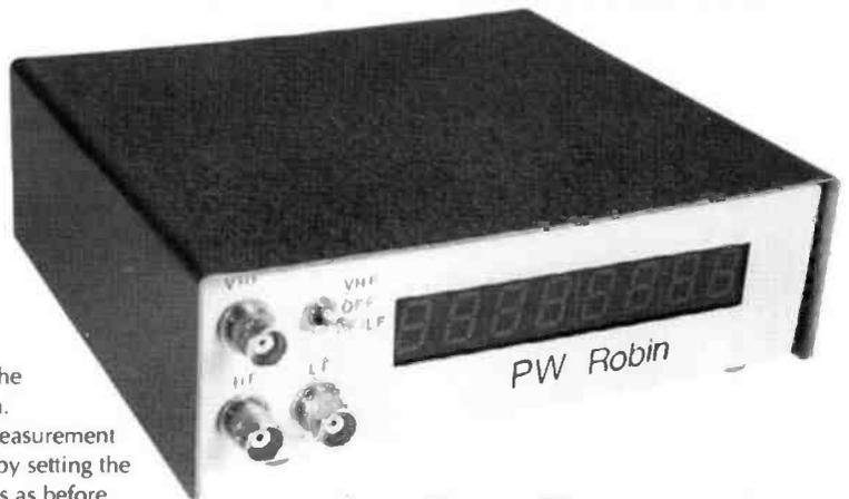
The additions I'm describing in this article extend the facilities on the PW Robin frequency meter, originally published in PW July 1991. My modifications add the facilities to measure both time and capacitance.
