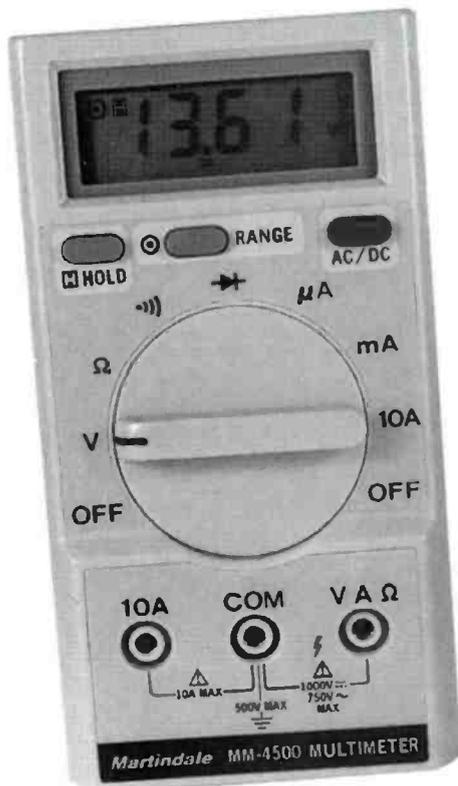
The Martindale MM-4500 digital multimeter has a three range ammeter from 0.1mA to 10A.
