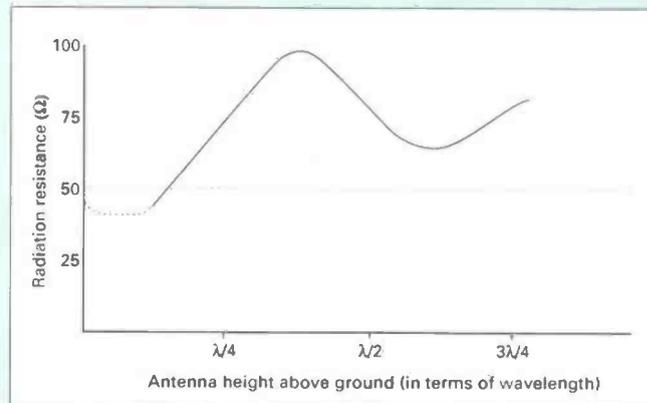
**Fig. 1: The radiation resistance of a  $\lambda/2$  dipole antenna varies with its distance above ground. When less than  $\lambda/8$  above ground this value is very unpredictable and depends greatly on the resistivity of the ground itself.**
