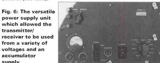
Fig. 6: The versatile power supply unit which allowed the transmitter/receiver to be used from a variety of voltages and an accumulator supply.
