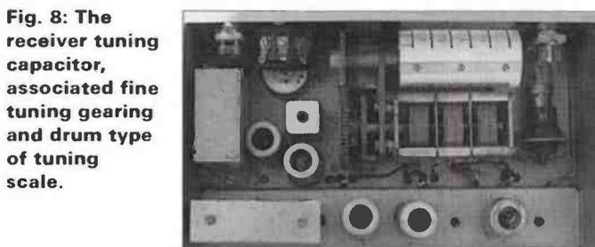
Fig. 8: The receiver tuning capacitor, associated fine tuning gearing and drum type of tuning scale.
