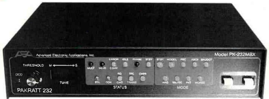
Since the inception of AEA's PK-232 TNC, there have been quite a few improvements. In this new form the multi-mode TNC comes complete with a variety of cables. There's a serial cable with DB25 connectors, two separate radio connector cables and a package to help set up the TNC. It also has a comprehensive operating manual.
