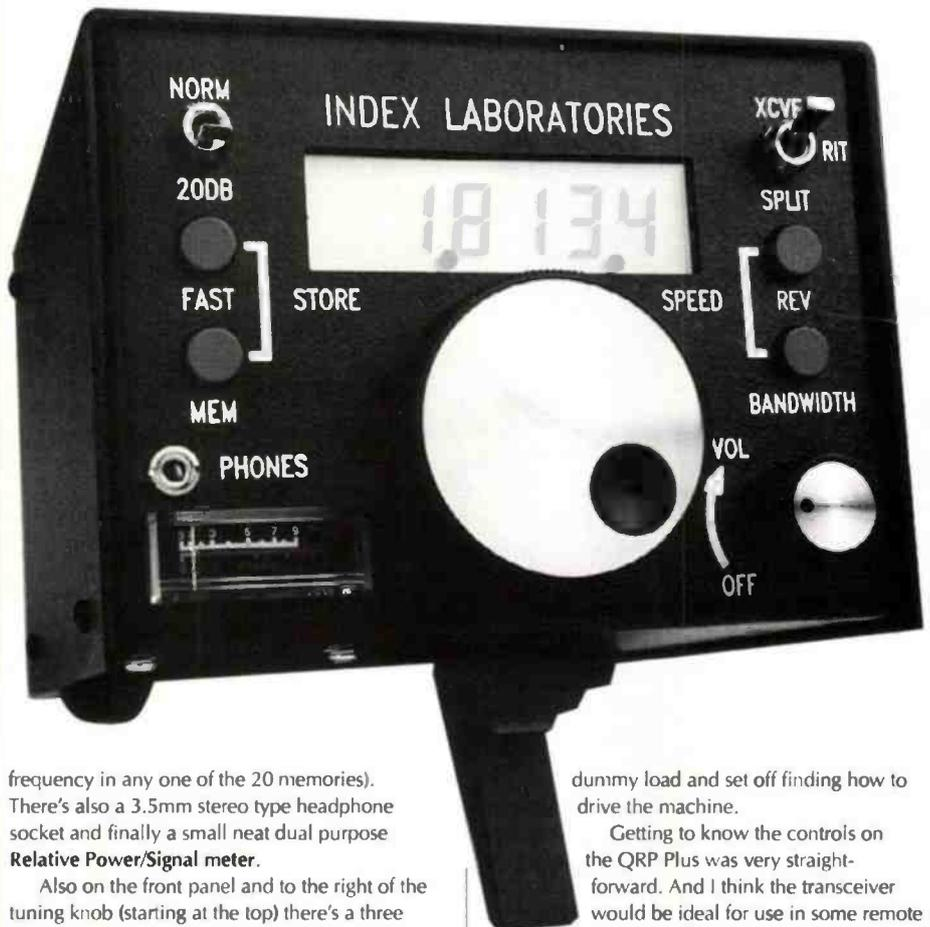
frequency in any one of the 20 memories). There's also a 3.5mm stereo type headphone socket and finally a small neat dual purpose **Relative Power/Signal meter**.
