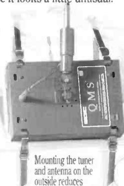
Mounting the tuner and antenna on the outside reduces engine noise and eliminates power-draining antenna wire runs between the antenna and tuner.
