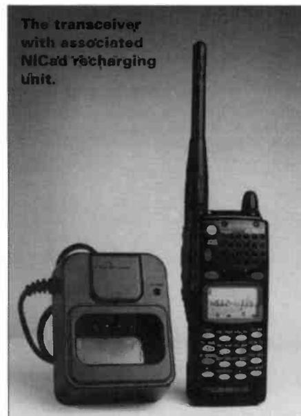
The transceiver with associated NiCad recharging unit.
