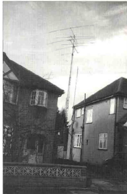
**Fig. 2: Don McLean G3NOF, based in Yeovil, Somerset, has been reporting on h.f. operations to PW for many years. The photograph shows Don's (top of tower) TET HB33SP 3-element, middle is the Tonna 9-element for 144MHz and bottom is the Cushcraft A3WS 3-element antenna. Don's trapped dipole can also be seen mounted on the pole on the side of his house.**
