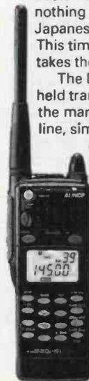
The DJ-191 is a v.h.f. f.m. hand-held transceiver and is described by the manufacturers as being "slim-line, simple to operate with its enormous display and effortless to use, large DTMF keypad". The frequency coverage is 144 - 145.995MHz with a maximum of 5W output.
