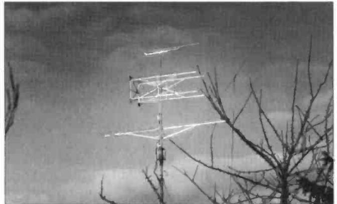
Here's a shot of the antenna system belonging to Ian Vincent G4MLY, secretary of the Kent Television Group. Top of the pole is a 44-element loop Yagi for 13cm; the receive converter is mounted here as well. Below are four 28-element loop yagis for 1296/1270MHz operation. All these are home-made, also the four-way power splitter. Closest to ground is the 13-element Tonna antenna for 144MHz. The whole system is mounted on a 28ft tall ex-Government mast and well guyed with 16 steel ropes.
