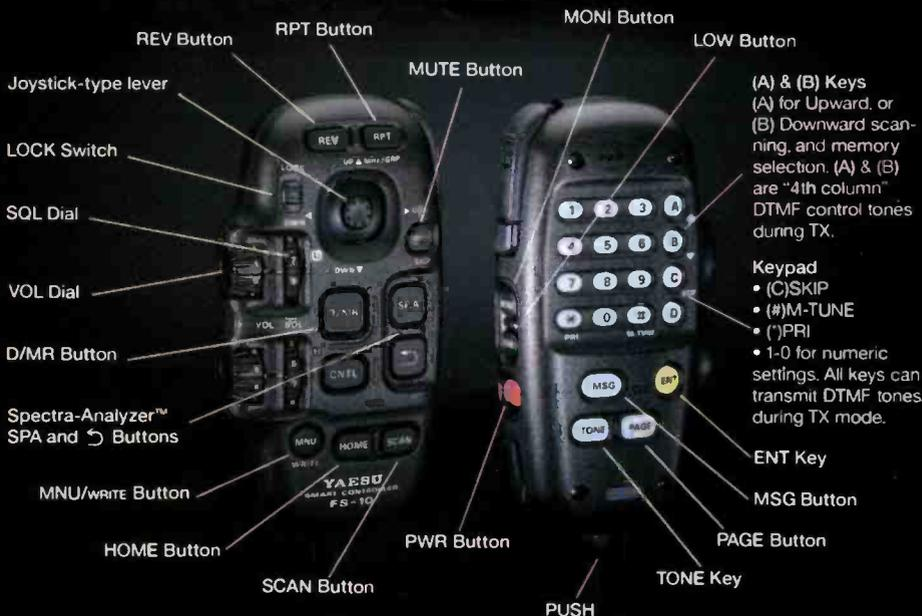
The FT-8500 and Smart Controller™ Microphone demonstrates Yaesu's world leadership position in 2-way radio communication again! With just four simple flicks of the Smart Controller™ Microphone "joystick"-type lever, you command over 50 separate functions from the palm of your hand! The FT-8500 defines "high-tech" in mobile radio engineering.
