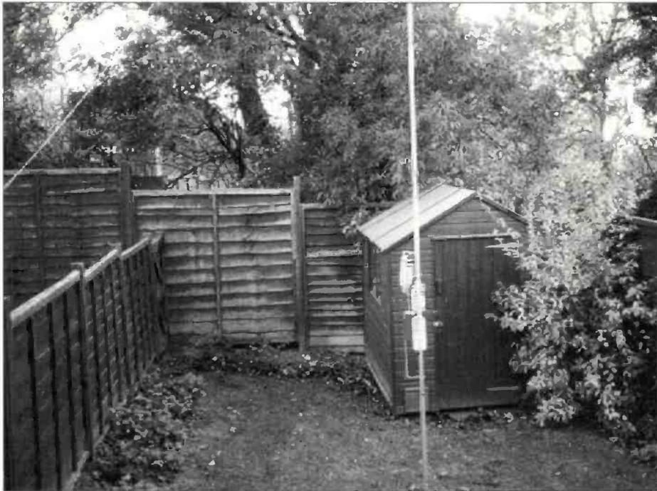
**The garden of the QTH at Hastings used on weekdays for two years by G4BUE. The 'postage stamp' sized back garden was just big enough to put up a Butternut HF6V vertical antenna, (3.5, 7, 10, 14, 21 and 28MHz) which with 100W from a TS-440 enabled Chris to keep up his DXing.**
