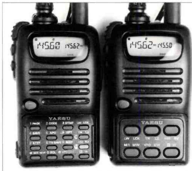
Photograph illustrating the choice of keyboards available on the FT-10R (see text).
