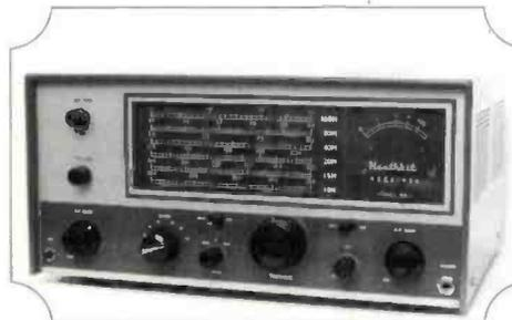
**Fig. 1: The Heathkit RA-1 amateur bands only communications receiver.**
