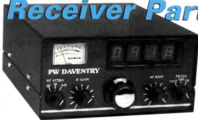
The Daventry's p.c.b. assembly is quite straightforward in concept. There's no coil winding or any special procedures, other than to observe static handling precautions with the dual-gate MOSFETS (BF981).
