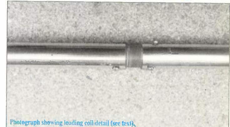
Photograph showing loading coil detail (see text).
