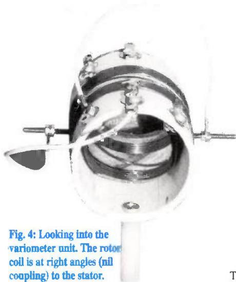
**Fig. 4:** Looking into the variometer unit. The rotor coil is at right angles (nil coupling) to the stator.
