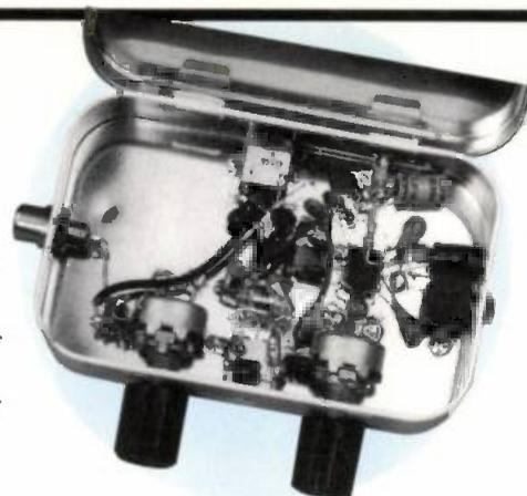
Inside view of the FF-7 receiver (in this version built into an 'Altoids' tin but a 'Fisherman's Friend' tin is the same physical size). George left the space for possible modifications or the inclusion of a small transmitter (see text).
