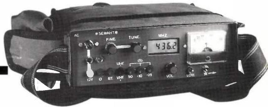
Recently I've been enjoying testing the portable Semaht u.h.f./v.h.f. digital field strength meter. It's a British made device marketed by Aerial Techniques of Poole in Dorset.
