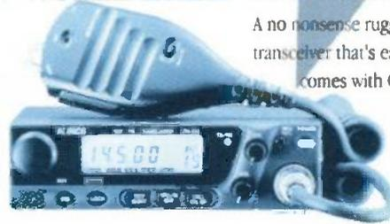
A no nonsense rugged 50W 144MHz mobile transceiver that's easy to use on the move and comes with CTCSS as standard
