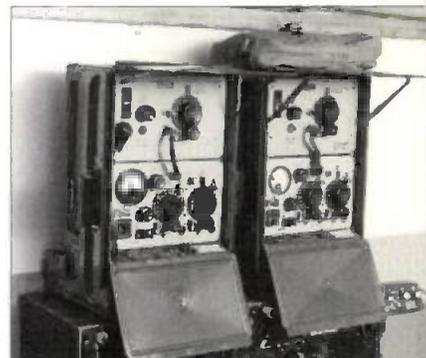
**Fig. 6: A pair of Wireless sets No. 18. The separate (removable for servicing) receiver unit is on top, with the separate transmitter (linked by an inter-unit plug and socket arrangement) at the bottom. The large combined h.t., bias and l.t. 'all dry' battery is housed inside the bottom unit, under the transmitter.**
