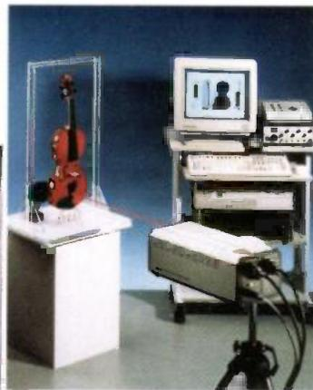
Photographs of a He:Ne laser scanning vibrometer installation being used to investigate the vibration pattern of a violin, and the resultant pattern.
