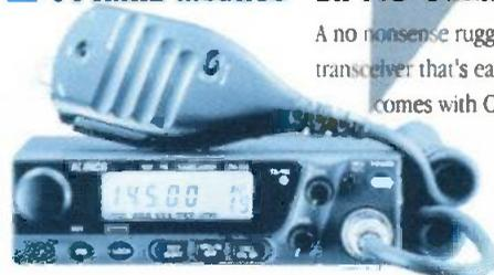
A no nonsense rugged 50W 144MHz mobile transceiver that's easy to use on the move and comes with CTCSS as standard
