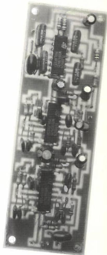
incoming audio from the receiver at line level is fed to C1, which acts as a d.c. 'blocking' capacitor and then to IC1, a quad operational amplifier.
