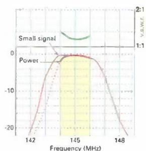
**Fig. 7: Out of band rejection and s.w.r. curves for the DC1-145-2H filter.**
