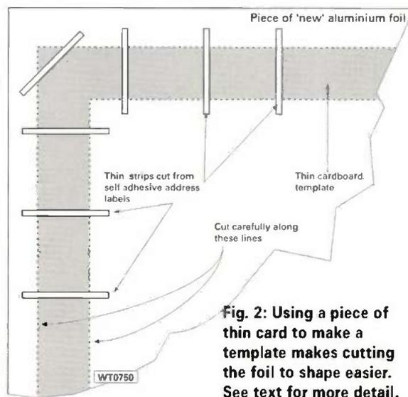
Fig. 2: Using a piece of thin card to make a template makes cutting the foil to shape easier. See text for more detail.
