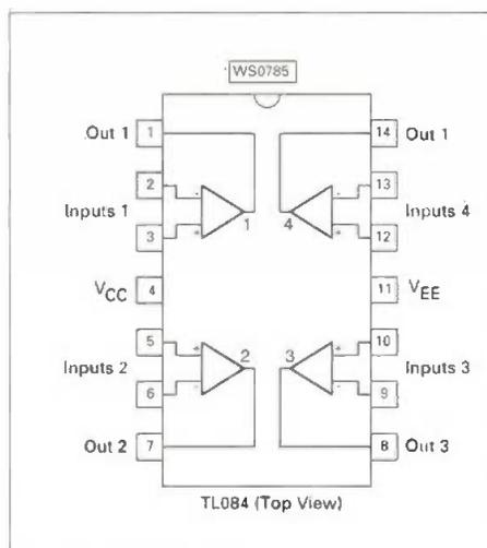
Fig. 5: Pin-out details of the TL084CN i.c. used for the project.
