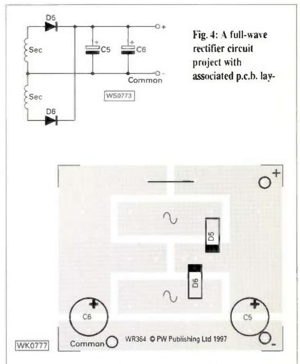
Fig. 4: A full-wave rectifier circuit project with associated p.c.b. lay-out.
