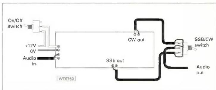
Fig. 4 Interconnections from p.c.b. (see text for suggestions on installation procedure for receiver to be used).
