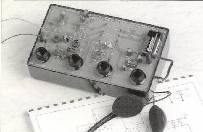
The manual contains complete schematics and theory of operation of all the building blocks. Use this trainer to receive frequencies from 500kHz to 110MHz!
