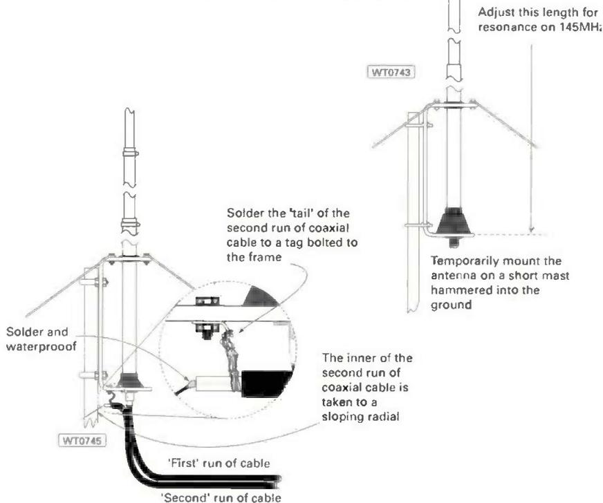
**Fig. 5:** A little more detail of how the second coaxial cable is attached. The connection within the dotted circle should be completely waterproofed with a bath sealant or similar.
