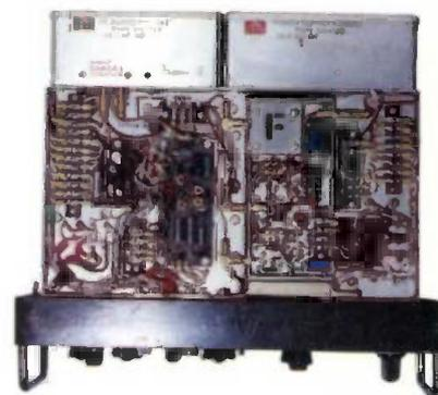
Again...the GR-345 is not really 'standing on its head'! This photograph shows the various unit interconnections and how small gold-plated plug and sockets route the r.f. signal through the various units.
