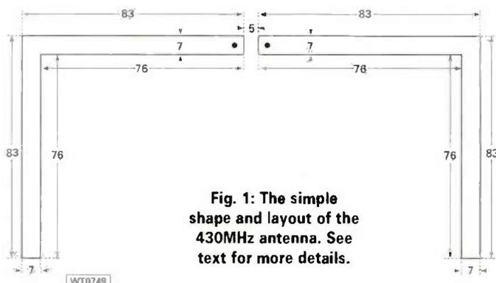
Fig. 1: The simple shape and layout of the 430MHz antenna. See text for more details.
