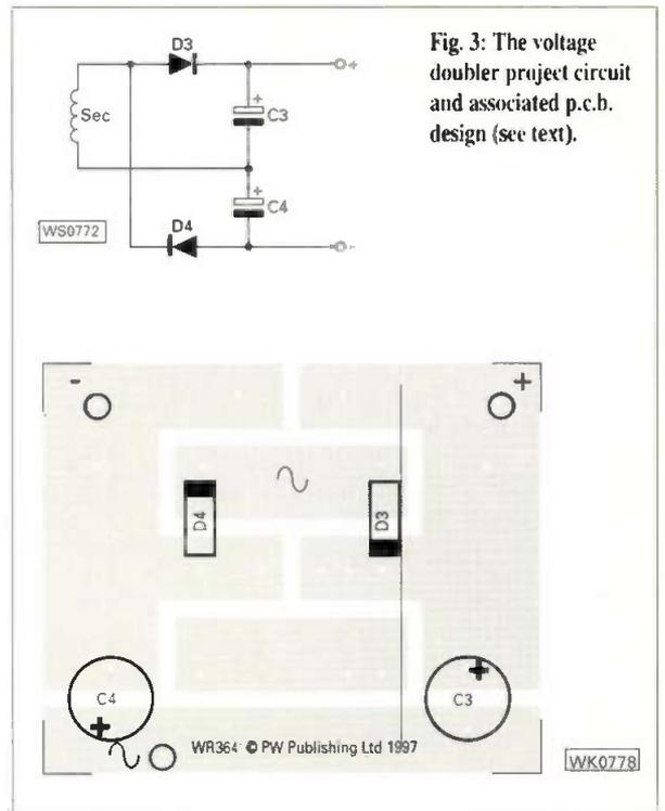
Fig. 3: The voltage doubler project circuit and associated p.c.b. design (see text).
