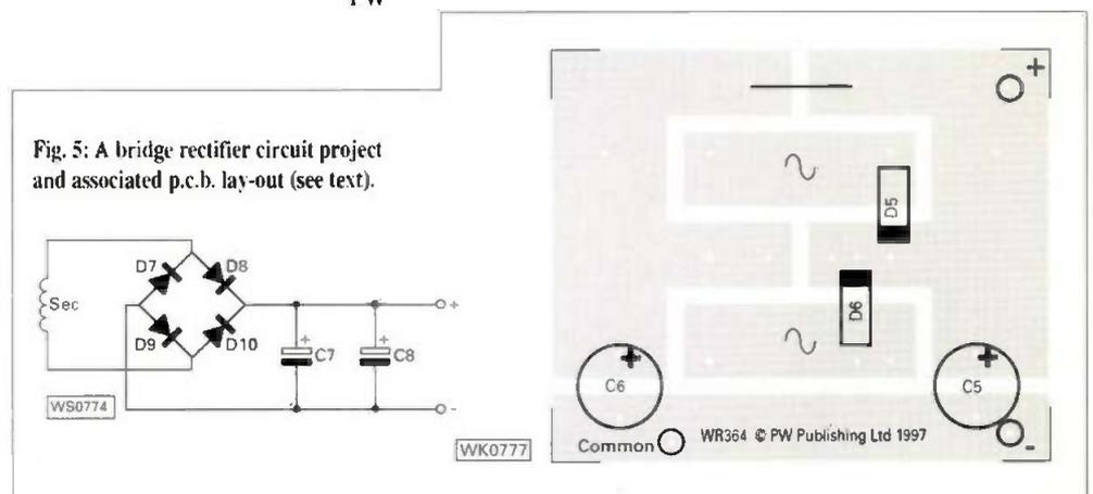
Fig. 5: A bridge rectifier circuit project and associated p.c.b. lay-out (see text).
