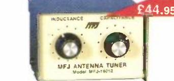
Covers 1.8MHz to 30MHz and matches any random wire to your hf transceiver. Handles 300 Watts and fitted SO-239. Ideal for portable work.
