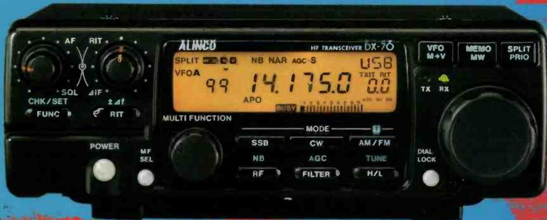
The DX70 TH packs a hefty 100W punch on all Ham bands 1.8 - 50MHz. It is backed by a superb receiver with narrow filters fitted as standard. Make no mistake - this is a real DX operators transceiver ideal for use at home, in the car, or for that portable DX-pedition. General coverage receive is included and wideband transmit facilities for export customers. The detachable front panel allows remote mounting and additional security.
