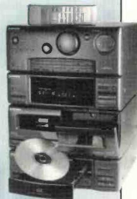
The Pioneer SX-P530 system features a stereo receiver (amplifier and synthesised tuner), twin cassette deck and CD player. It comes complete with two 60W 8Ω speakers, remote control unit, f.m. and a.m. antennas and full operating instructions.
