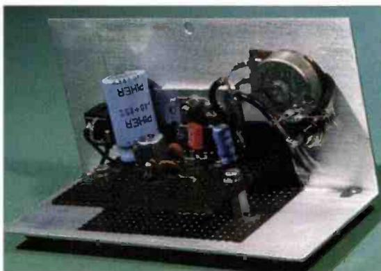
photograph, **Fig. 4**, is built on Veroboard. It lays out very well in this medium. The only slight quirk is that the decoupling capacitor is mounted under the board.
