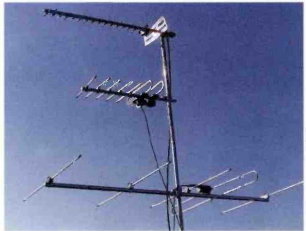
Antennas used by Graham Hankins G8EMX for portable ATV contests. From top: 24, 70cm and 2m for ATV calling. Note: even the 2m antenna is mounted horizontally. Larger antennas would be preferable.
