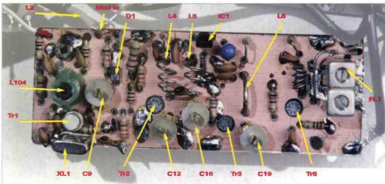
Fig. 3: The transmitter board overlay.
