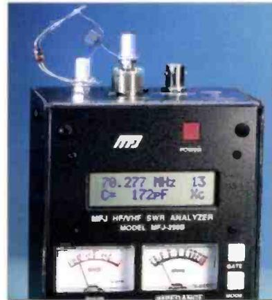
Fig. 4: The 13Ω reactive impedance of Fig. 3, might be a 172pF capacitor...
