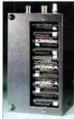
Fig. 1: A newly engineered battery box holding 10 AA cells or NiCad rechargeable batteries. A jumper (switch) is used to enable the automatic charging circuit.
