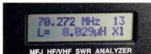
Fig. 5: ...or it might be an inductance of 29nH. Only further tests will establish what it actually is.
