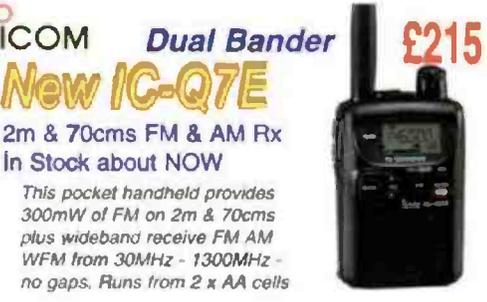
This pocket handheld provides 300mW of FM on 2m & 70cms plus wideband receive FM AM WFM from 30MHz - 1300MHz - no gaps. Runs from 2 x AA cells
