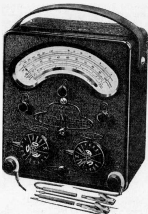
FIG. 11.—Above is one of the popular Avometers, designed for A.C. or D.C. use.
