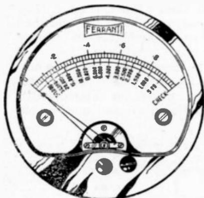
FIG. 29.—Showing the resistance calibrated readings added to the scale of a milliammeter.
