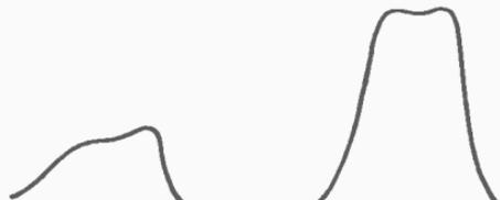
FIGS. 135 and 136.—On the left is seen the effect of heavy damping on an I.F. circuit, and on the right how it appears when the damping is removed.
