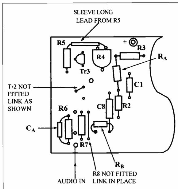
Fig. 8: Modifications to the Velleman P1771 FM transmitter module - see Figs. 4/5 and Table 2.
