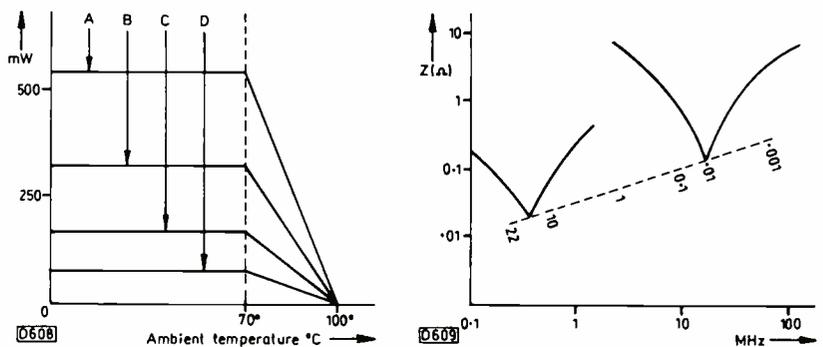
**Fig. 2 (left): Maximum permissible power dissipation for various capacitor body sizes. A 15.5mm thick, 27.5mm pitch; B 11mm thick, 22.5mm pitch; C 8.5mm thick, 15mm pitch; D 4.5mm thick, 10mm pitch.**
