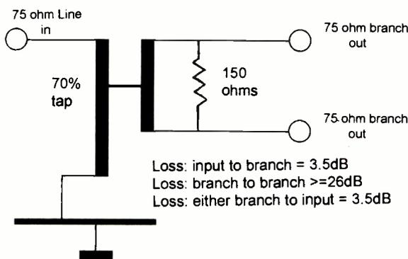
Fig. 3: A two-way equal splitter circuit.
