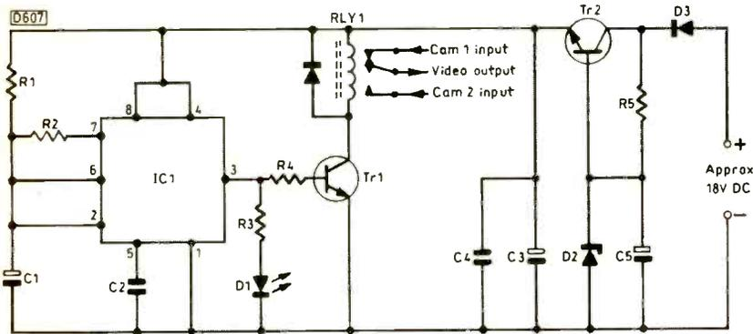
Fig. 1: Circuit diagram of the scart switcher unit. The video inputs and the output (flying lead) are all connected to pin 20 of the relevant scart connector.
