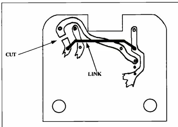
Fig. 7: The cut-and-link modification on the print side of the power supply PCB.
