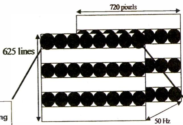
Fig. 2: The two different DRC-MF modes, DRC50 and DRC100. Note that the drawing does not show correct 625-line signal interlacing.
