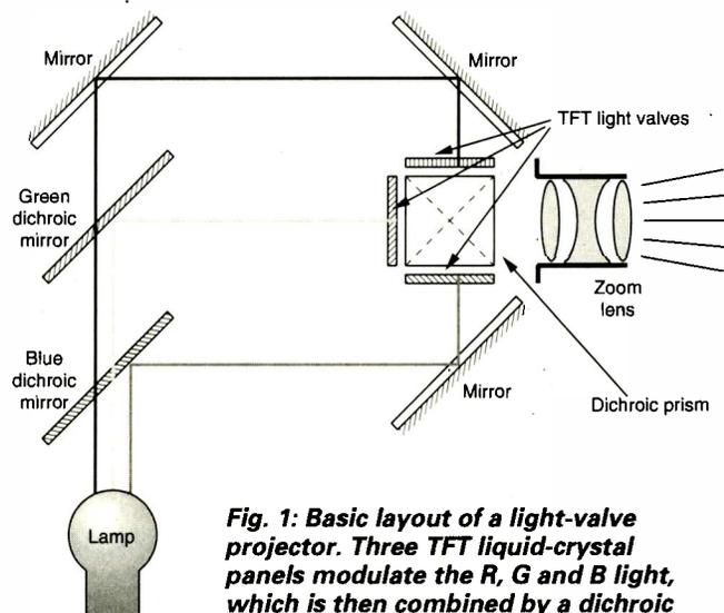
**Fig. 1: Basic layout of a light-valve projector. Three TFT liquid-crystal panels modulate the R, G and B light, which is then combined by a dichroic prism.**
