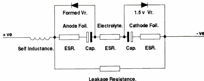
**Fig. 1. Equivalent circuit of a polarised aluminium electrolytic capacitor. The cathode foil is etched but not formed. Its natural atmospheric oxide equates roughly to 1.5V of electrical formation. Using similar foil thickness and etch ratio as the anode foil, a 6V rated capacitor's cathode capacitance will exceed that of the anode by a good margin, but CV products will be similar.**
