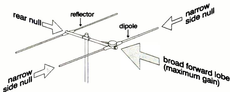
Fig.5. An array mounted horizontally has side nulls because a dipole is very insensitive to signals arriving 'end on'. The side nulls are deep, but very accurate alignment is required to make use of them.
