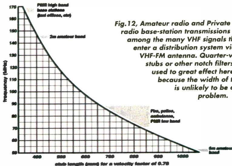
**Fig. 12.** Amateur radio and Private Mobile radio base-station transmissions are among the many VHF signals that can enter a distribution system via the VHF-FM antenna. Quarter-wave stubs or other notch filters can be used to great effect here, because the width of the notch is unlikely to be a problem.
