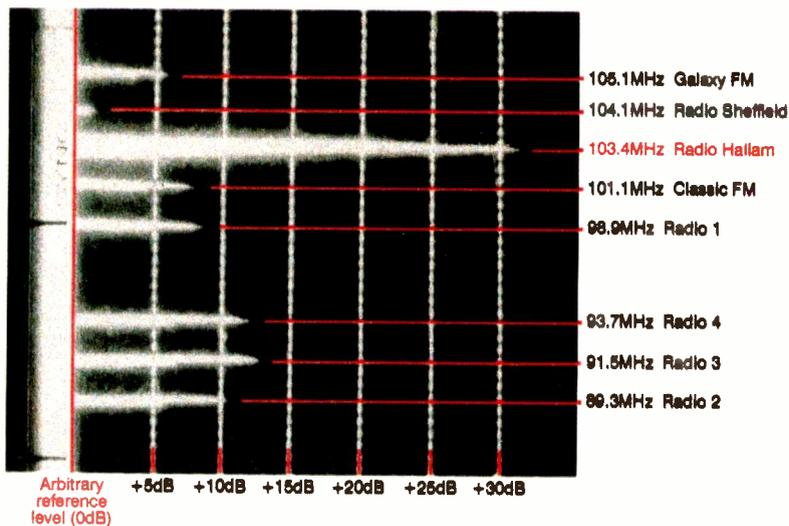
**Fig. 10. Antenna feed as in Fig. 9, but with  $1/4$ -wave stub tuned to 103.4MHz. Signal at 103.4MHz has dropped 24dB. At 104.4MHz, 7 channels higher, it has lost 15dB. At 96.9MHz, 22 channels lower, it is -10dB. This sounds bad, but the notch means that antenna output enters the distribution amplifier 20dB up, which lifts signals 5dB, or so, further above the noise floor.**
