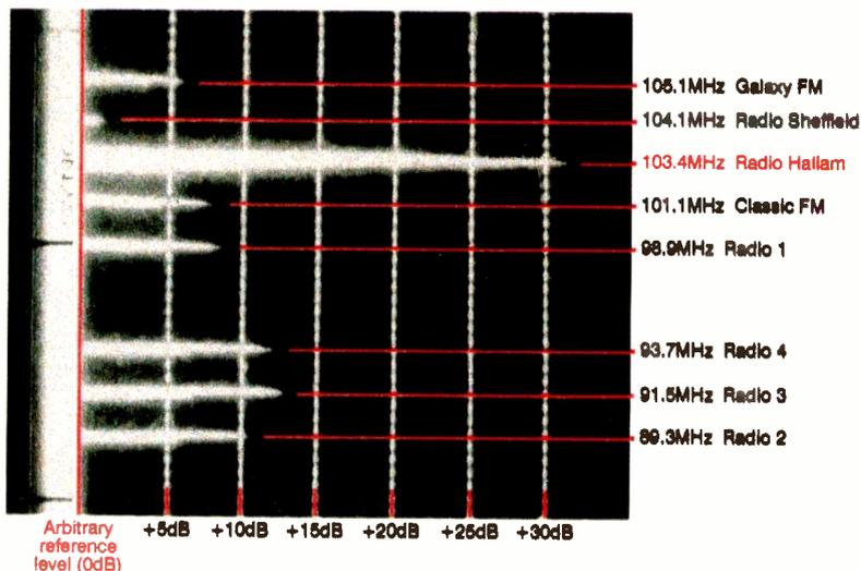
**Fig. 10. Antenna feed as in Fig. 9, but with  $\frac{1}{4}$ -wave stub tuned to 103.4MHz. Signal at 103.4MHz has dropped 24dB. At 104.4MHz, 7 channels higher, it has lost 15dB. At 96.9MHz, 22 channels lower, it is -10dB. This sounds bad, but the notch means that antenna output enters the distribution amplifier 20dB up, which lifts signals 5dB, or so, further above the noise floor.**
