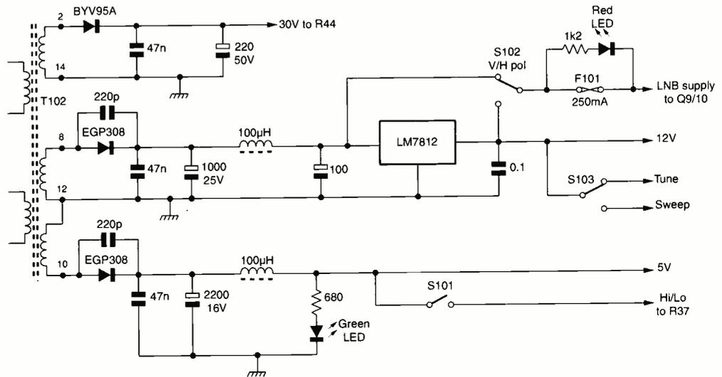
Fig. 3: Circuitry on the secondary side of the power supply.
