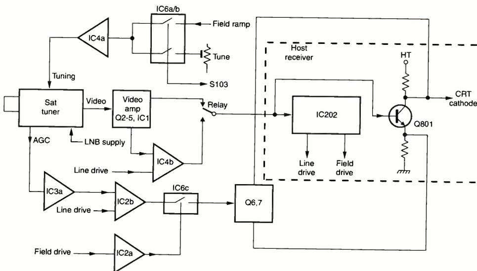
Fig. 1: Block diagram of the satellite band scanner.
