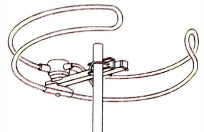
**Fig. 4.** The common 'halo' VHF-FM antenna is omni-directional and horizontally polarised but its gain is very poor.
