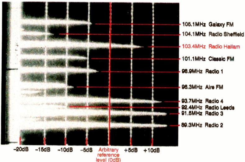
so to speak. The result is a deep notch in the response of the main transmission line. The quarter-wave stub is, in fact, a homemade notch filter. To find a quarter of a wavelength in cable:
