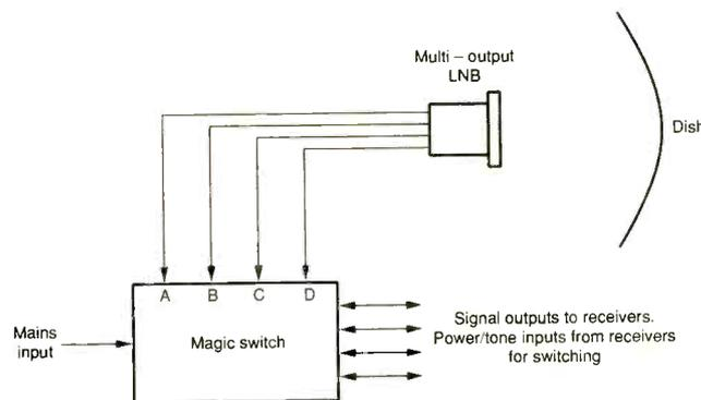
**Fig. 1: SMATV IF distribution system for use with Astra 2. The magic switch inputs are A high-band vertical, B high-band horizontal, C low-band vertical, D low-band horizontal. The LNB is continuously powered by the magic switch. The digibox power/tone outputs select the required band and polarisation at the magic switch.**
