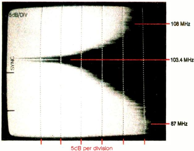
**Fig. 8. Spectrum display showing response notch obtained with a  $1/4$ -wave stub, centred on 103.4MHz in a workshop half a mile from a medium-power transmitter on that frequency. A tiny signal can be seen at the bottom of the notch. This has entered between the notch filter and the analyser despite the use of good screening techniques.**
