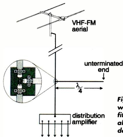
Fig.6. The quarter-wave stub can be fitted anywhere along the download.
