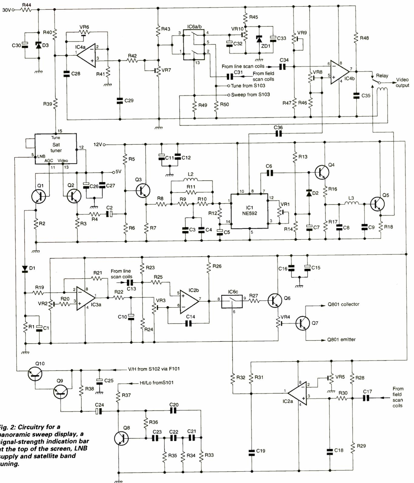
**Fig. 2: Circuitry for a panoramic sweep display, a signal-strength indication bar at the top of the screen, LNB supply and satellite band tuning.**
