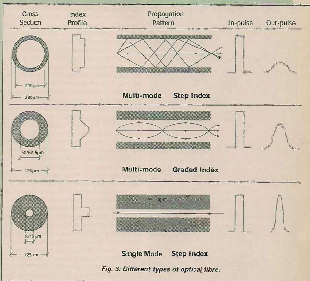
Fig. 3: Different types of optical fibre.
