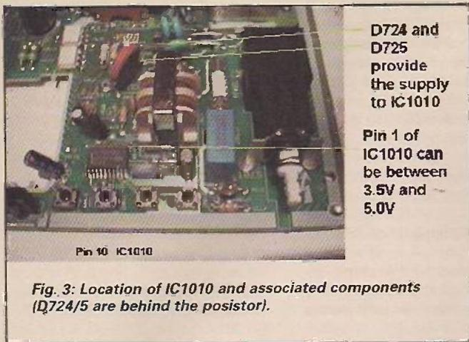
Fig. 3: Location of IC1010 and associated components (D724/5 are behind the posistor).
