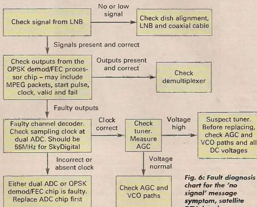
Fig. 6: Fault diagnosis chart for the 'no signal' message symptom, satellite DTV decoder.
