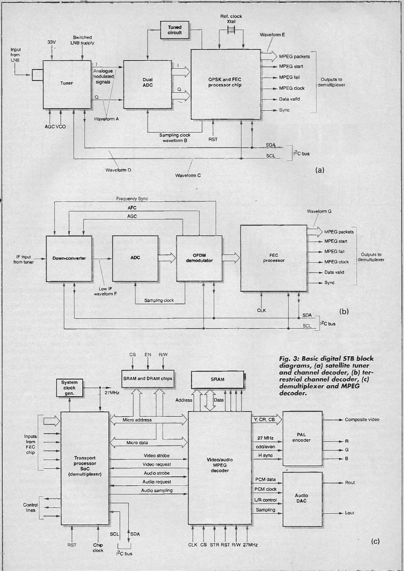
**Fig. 3: Basic digital STB block diagrams, (a) satellite tuner and channel decoder, (b) terrestrial channel decoder, (c) demultiplexer and MPEG decoder.**
