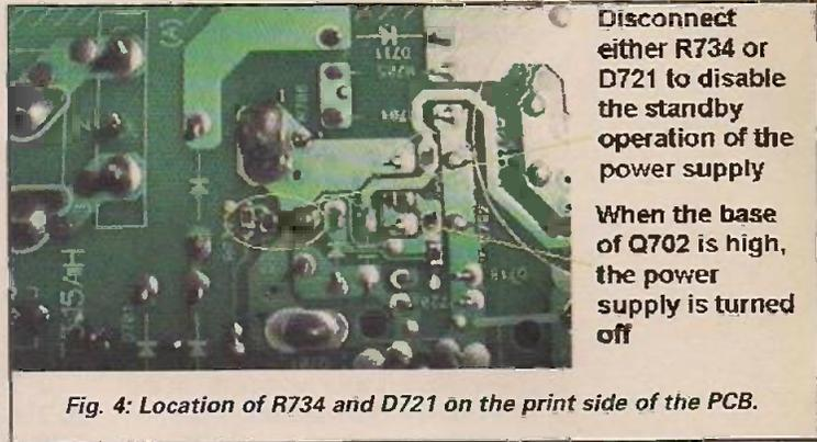
Fig. 4: Location of R734 and D721 on the print side of the PCB.
