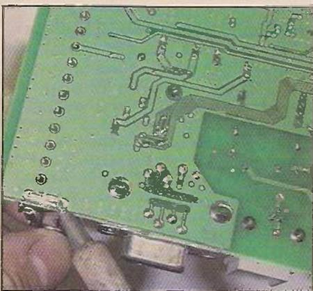
**Photo 2: Unsoldering the tuner module's lugs in the Amstrad DRX100 digibox.**
