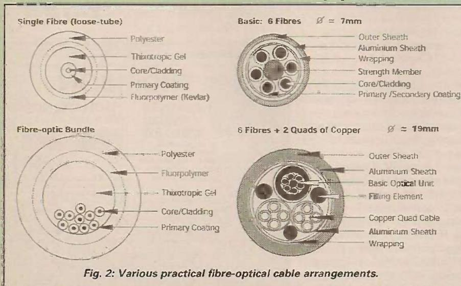
Fig. 2: Various practical fibre-optic cable arrangements.
