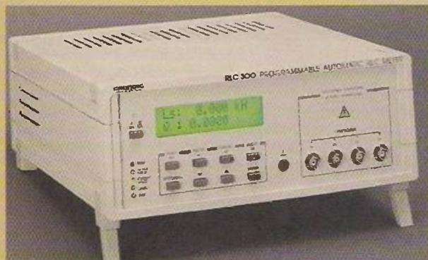
Vann Draper Electronics, world-wide distributor for Grundig Test Instruments, has introduced a range of three new automatic LCR meters. Model RLC300 is an automatic/manual instrument for professional applications, with eight measuring parameters, tolerance and relative results, level and phase, four test frequencies and two voltages for electrolytics and polarisation. Model RLC200 has a reduced specification and a basic resolution of 0.2%. With Model RLC100 the resolution is 0.5%.
