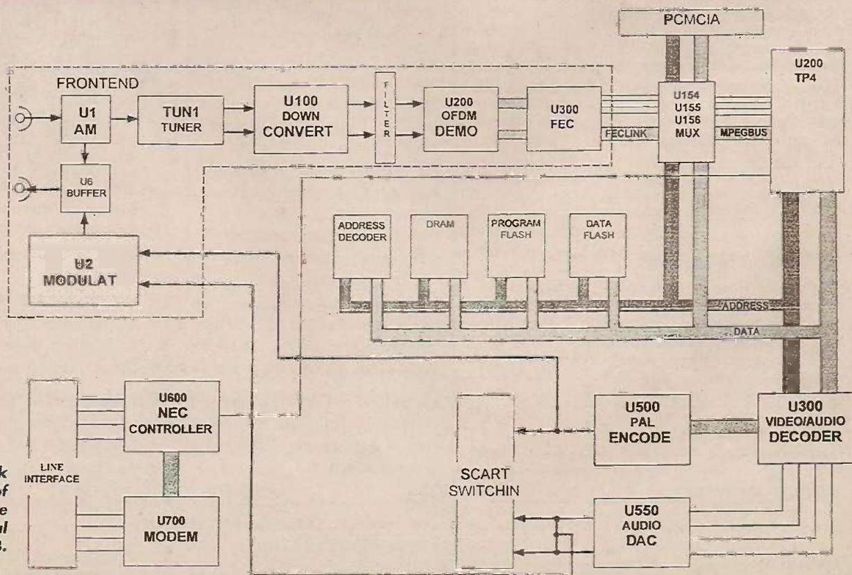
Fig. 2: Block diagram of the Pace ONdigital STB.
