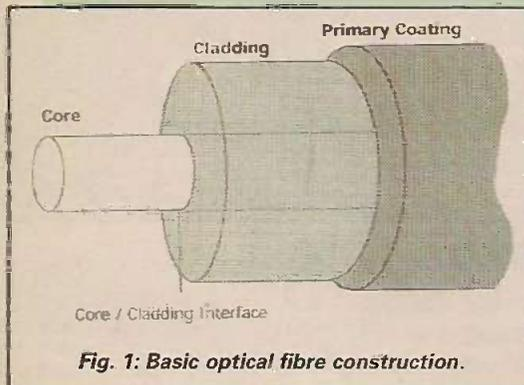
Fig. 1: Basic optical fibre construction.
