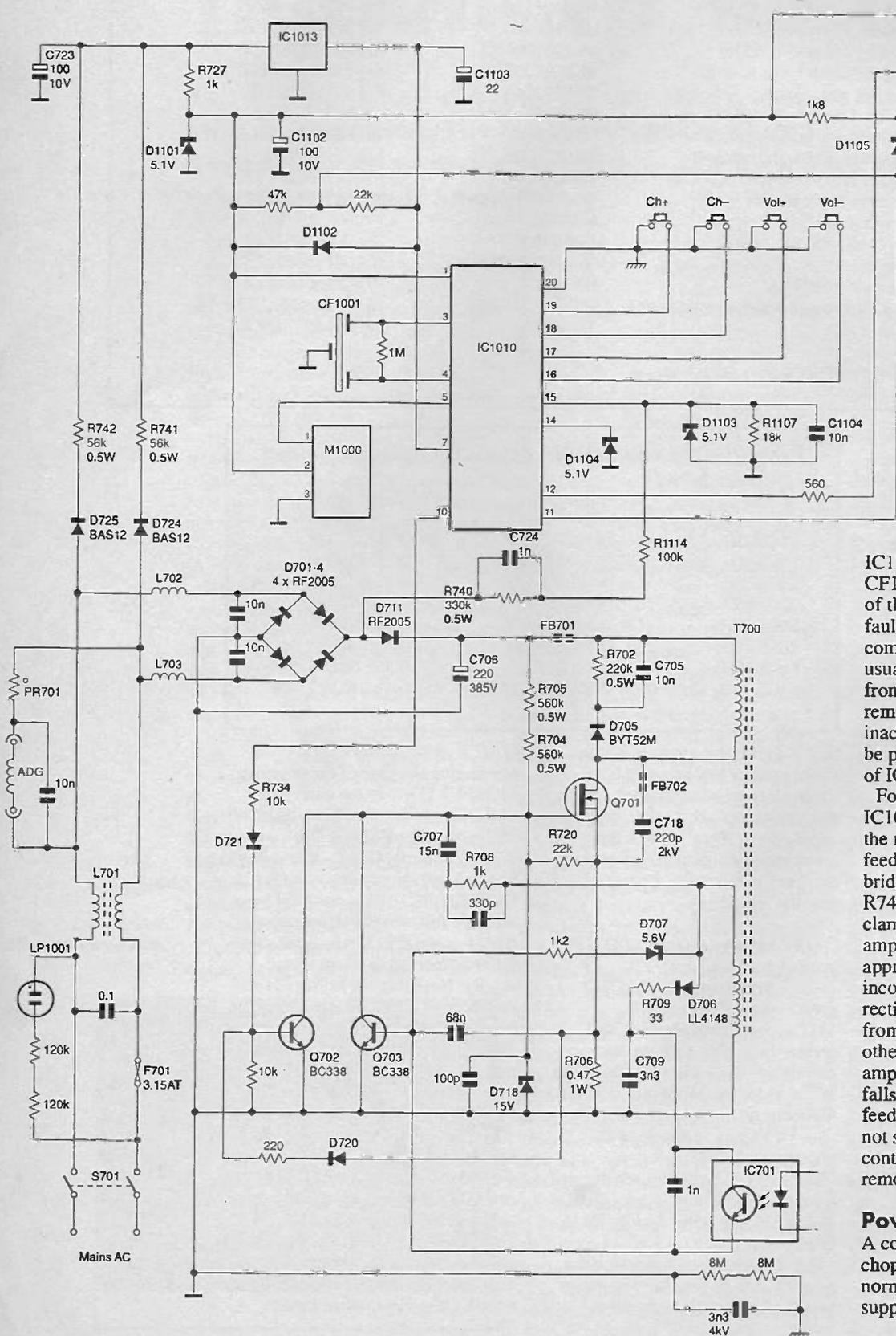
Fig. 2: Circuitry on the primary side of the chopper power supply. 59/66cm models have C733 (220p, 2kV) in parallel with C718 and R706 is 0-33Ω.
